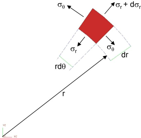
Now consider an element at radius  $r$  and defined by an angle increment  $d\theta$  and a radial increment  $dr$ . By circular symmetry, the stresses  $\sigma_\theta$  and  $\sigma_r$  are functions of  $r$  only, not  $\theta$  and the shear stress on the element must be zero. For an element of unit thickness, radial force equilibrium gives:
