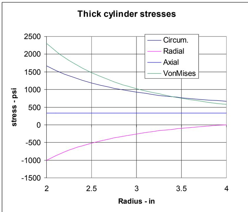
Example of cylinder with  $P_i = 1000$  psi,  $r_i = 2$ " and  $r_o = 4$ "
