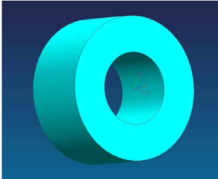
Consider a thick walled cylinder with open ends as shown above. It is loaded by internal pressure  $P_i$  and external pressure  $P_o$  as seen below. It has inner radius  $r_i$  and outer radius  $r_o$ .
