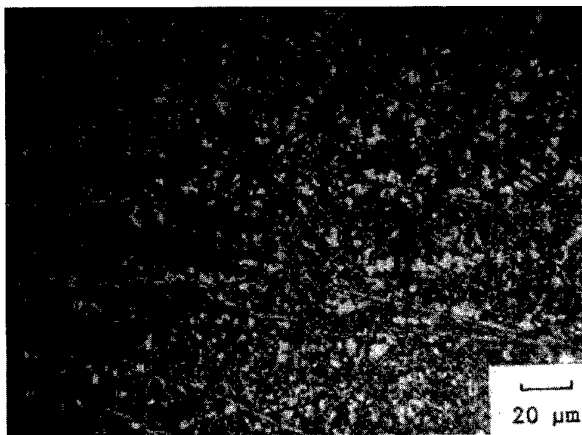
Figure 11 Wear track with PTFE transfer film on WC-Co counterface after 23 hours testing. Initial roughness 0.076μm
