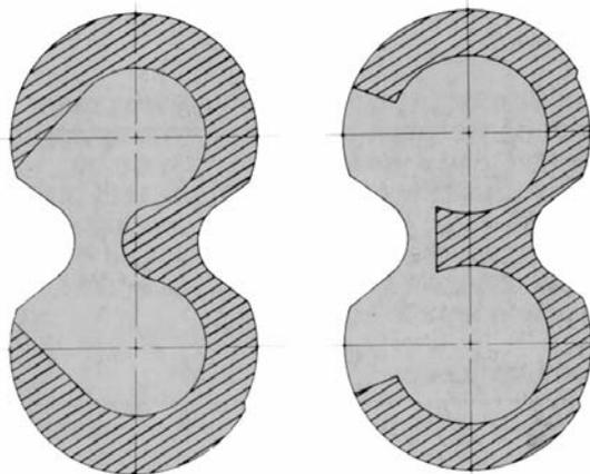
Area of pressure loading shaded (system pressure applied on rear faces of bearing blocks)
