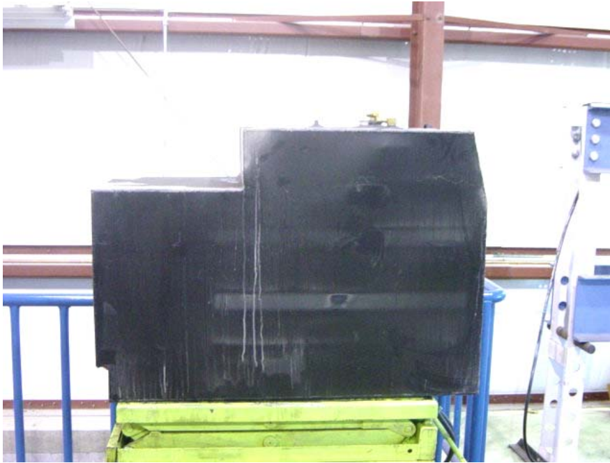
FUEL LEAKING FROM LEFT SIDE FUEL TANK (440 TEST MILES)
