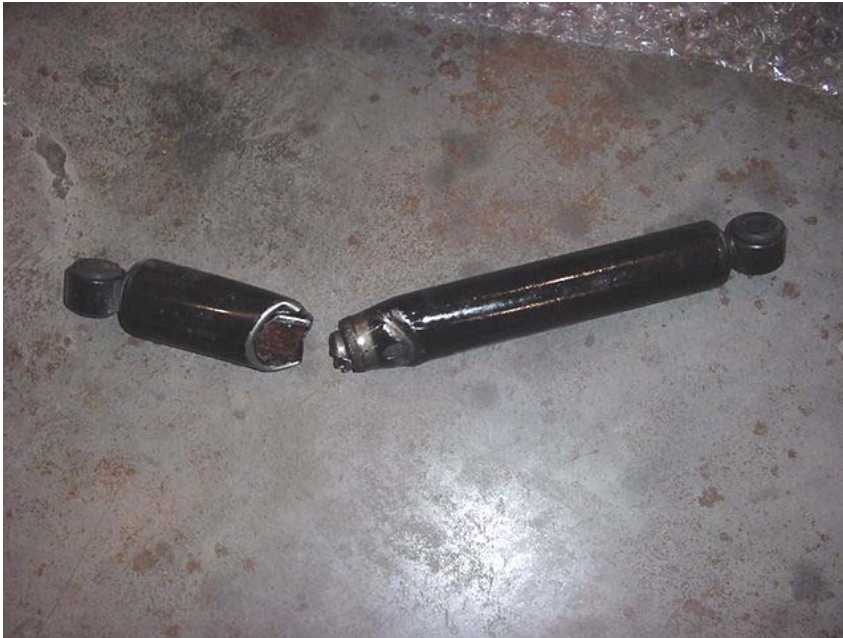
LEFT FRONT SHOCK PULLED APART (2,309 TEST MILES)
