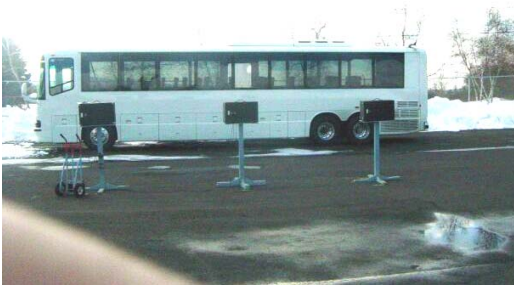
TEST BUS SET-UP FOR 80 dB(A) INTERIOR NOISE TEST
