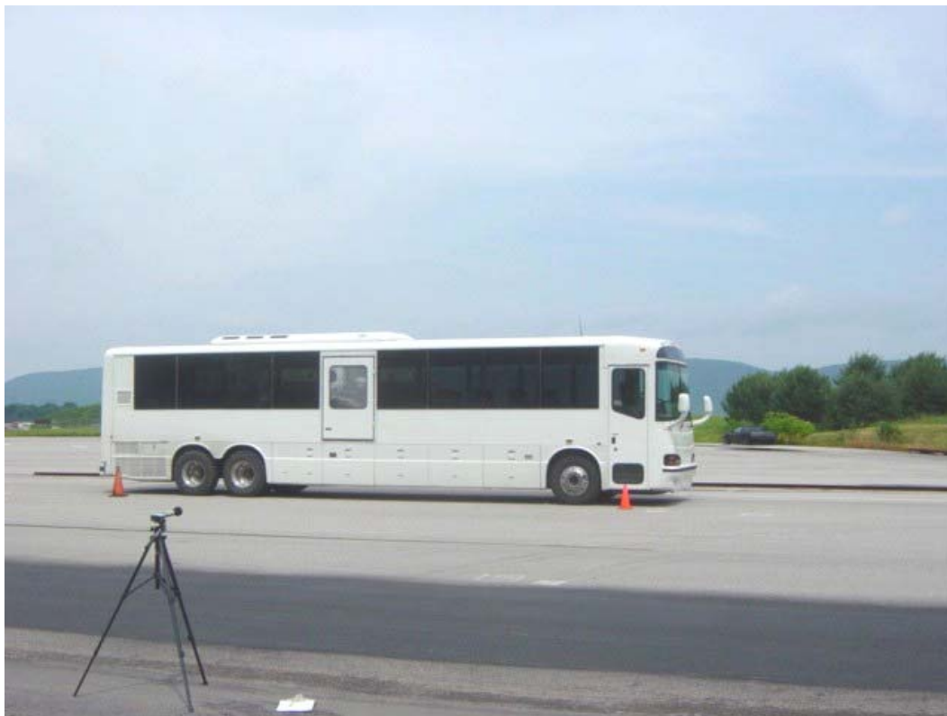
TEST BUS UNDERGOING EXTERIOR NOISE TESTING
