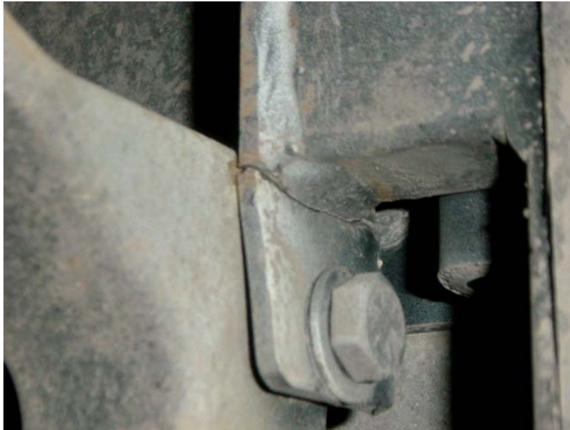
CRACKED FRAME WORK AT LOWER RADIUS ROD ATTACHMENT (1,809 TEST MILES)
