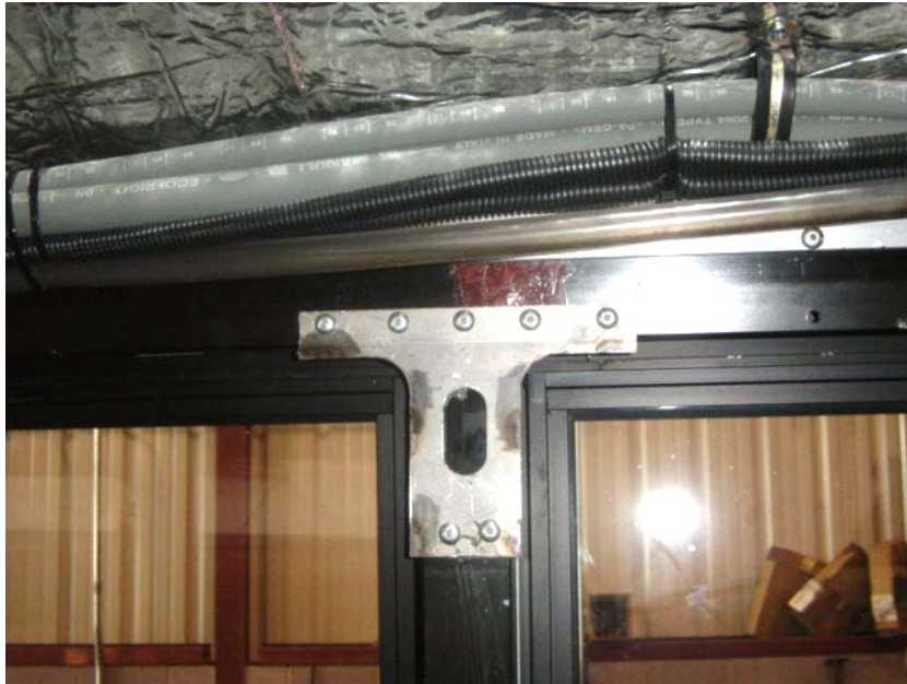
“T” GUSSETS ADDED AT THE TOP OF WINDOW JUNCTURES (8,106 TEST MILES)
