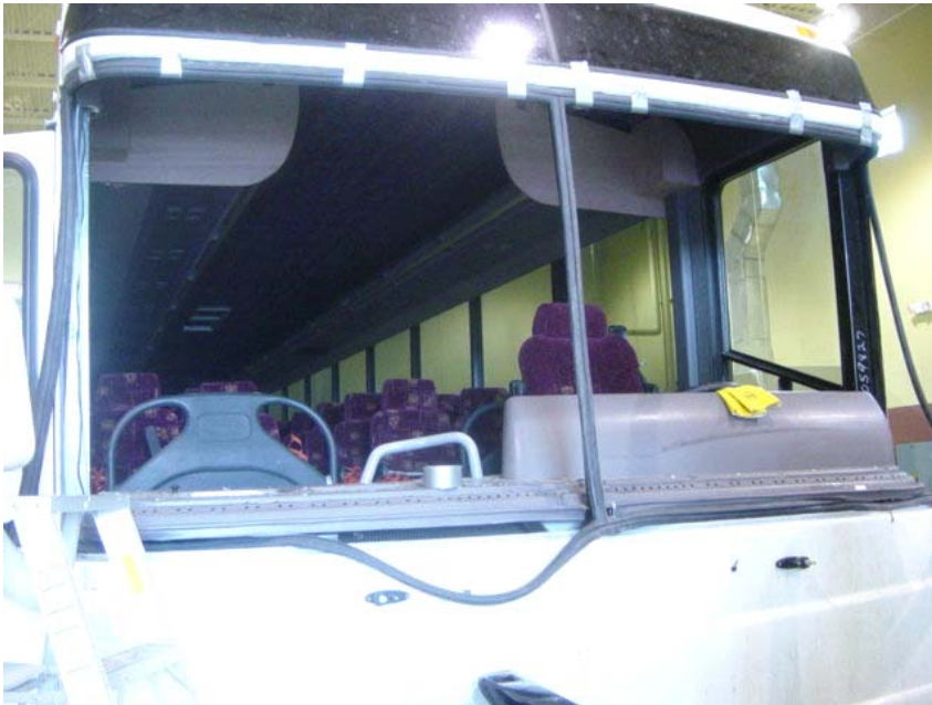
RIGHT SIDE WINDSHIELD FELL OUT (6,022 TEST MILES)
