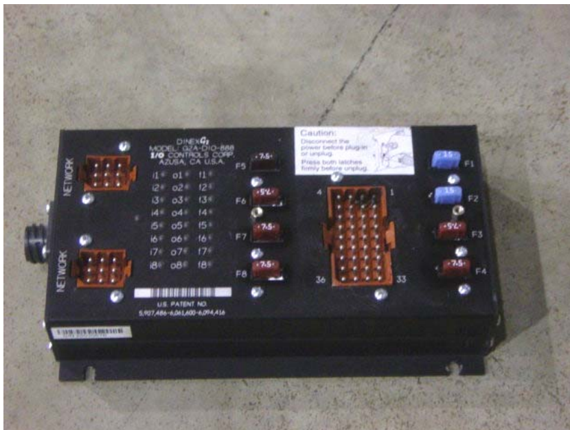
FAILED B1 MODULE (2,175 TEST MILES)
