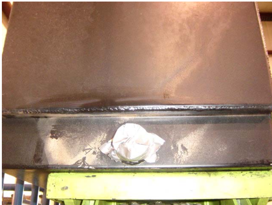
FUEL LEAKING FROM LEFT SIDE FUEL TANK (440 TEST MILES)
