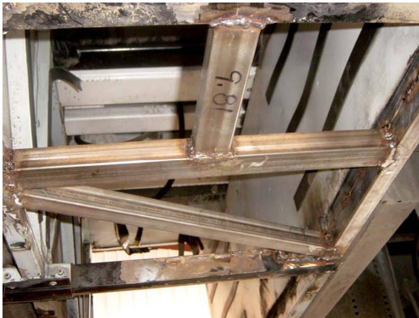
FRAME WORK ADDED NEAR RADIUS ROD MOUNTS (8,978 TEST MILES)
