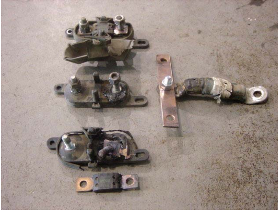
FAILED FUSE HOLDERS (14,439 TEST MILES)
