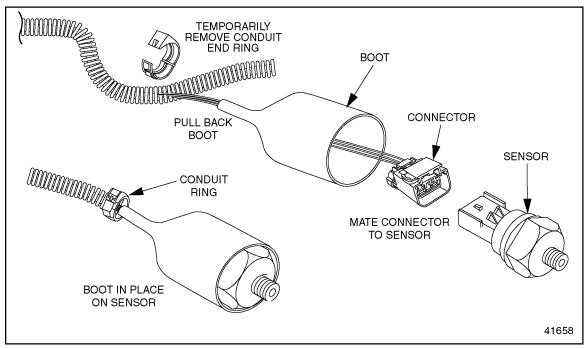
Figure 5. Exhaust Back Pressure Sensor with Sensor Boot
