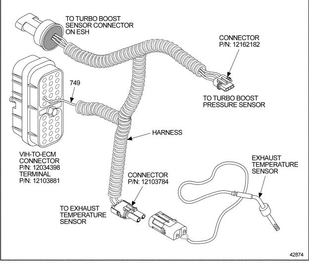
Figure 1. Exhaust Temperature Sensor Harness (to be removed)
