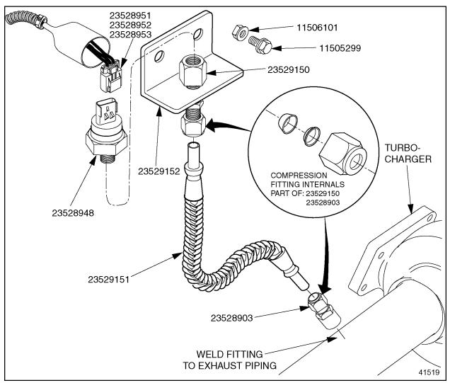
Figure 2. Installation of Exhaust Back Pressure Sensor Kit
