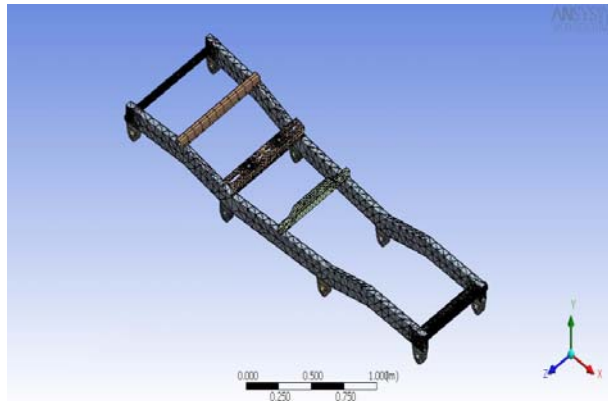
Figure 6.1: Truck chassis model meshed with tetrahedral -10 elements
