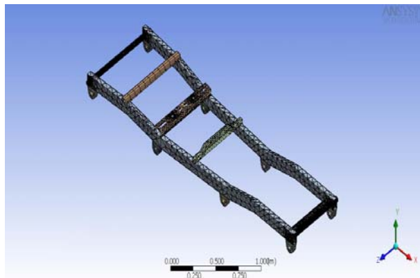
Figure 4.18: Truck chassis model meshed with tetrahedral -10 elements
