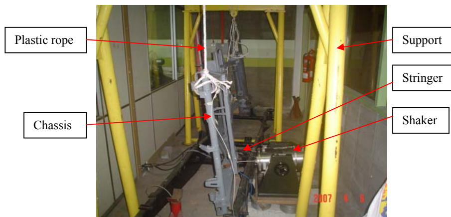
Figure 5.3: Shaker Test Set-up
