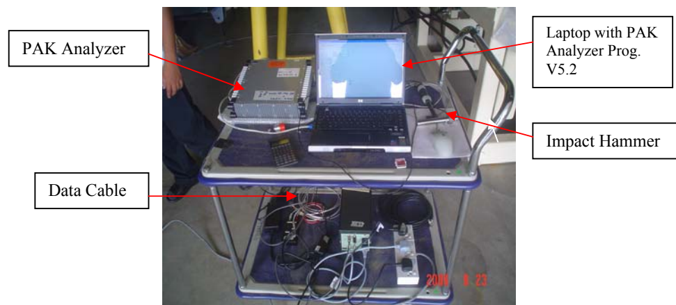
Figure 5.2: Experimental setup for impact hammer test.
