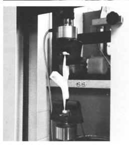
Tests for tear strength analyze both long term durability and the foam's ability to be handled during product assembly.
