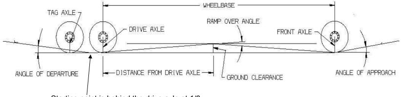
Starting point is behind the drive axle at 1/3 of the distance between the 2 rear axles.
