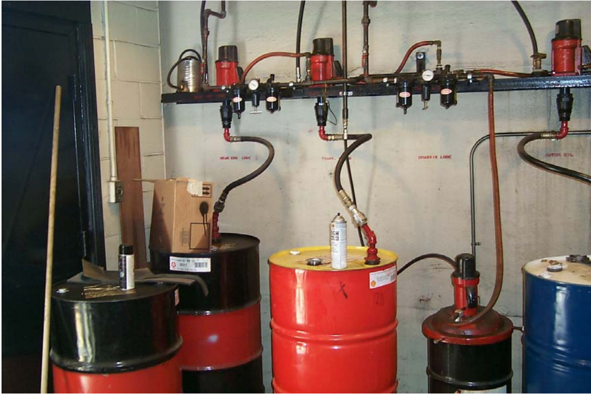
Fluids Room: Storage drums with pumps to overhead reels system
