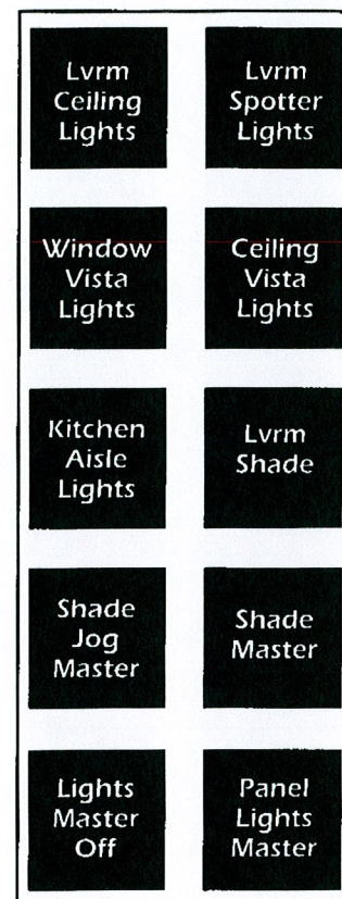
Sample of panel with shade controls. Buttons may vary according to model of coach ordered. Buttons work the same.
