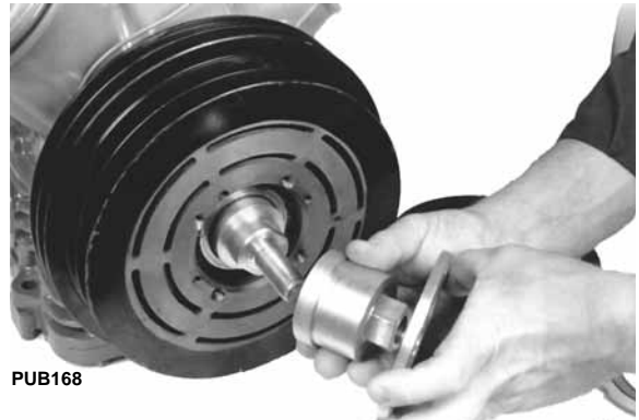
Figure 91: Installing Tool Body and Collar
