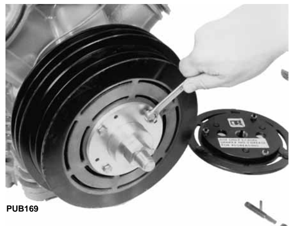
Figure 92: Securing Collar to Pulley
