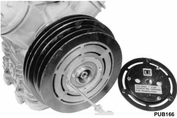
Figure 89: Removing Seal Assembly
