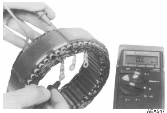
Figure 121: Test for Continuity Between Windings and the Laminations
