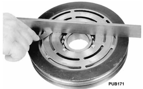
Figure 94: Checking for Warpage
