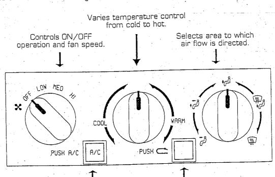
Activates compressor Engages recirculated for air conditioner air flow
