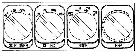
Turns the air conditioner compressor on or off and allows for recirculated air flow.
