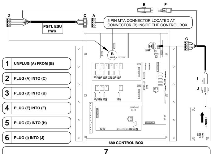
COMPLETELY REMOVE THE OLD SENSING UNIT AND IT'S HARDWARE. DO NOT USE THE OLD HOLES OR HARDWARE FOR MOUNTING THE NEW SENSING UNIT. MOUNT THE NEW SENSING UNIT IN THE SAME MANNER AS THE OLD ONE. "THIS SIDE UP" TEXT ON THE UNIT IS FACING THE SKY NOT THE GROUND. BE SURE THAT THE FRONT (ARROW) ON THE UNIT IS ORIENTED TO THE FRONT OF THE VEHICLE. PLUG THE HARNESS AND SENSING UNIT TOGETHER.
