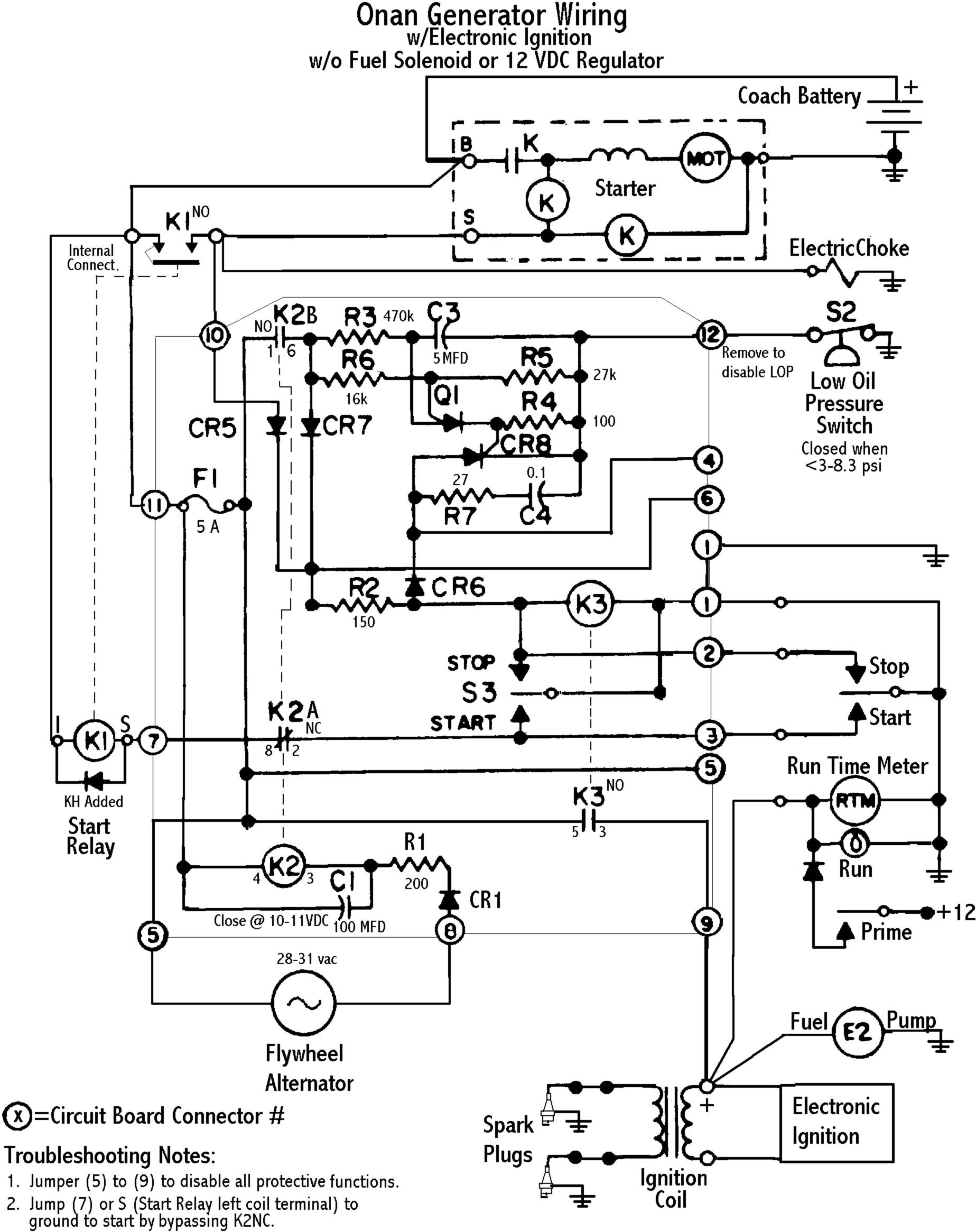
3. Jump (12) to Ground to test LOP stop within 3-4 sec.
