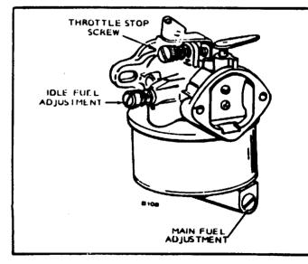
FIGURE 13. CARBURETOR ADJUSTMENTS
