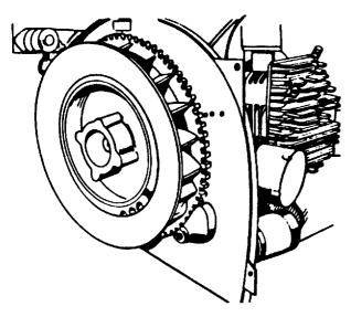
FIGURE 41. BLOWER SCROLL REMOVED
