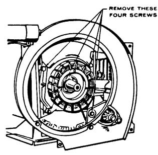
FIGURE 42. REMOVING BACKING PLATE
