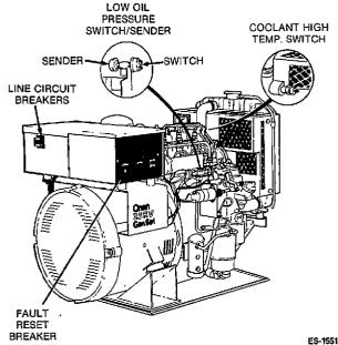
FIGURE 5. FAULT SENSOR LOCATION
