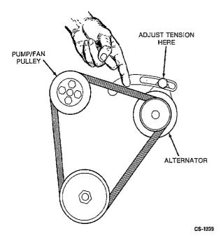
FIGURE 8. BELT TENSION ADJUSTMENT
