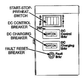
FIGURE 4. DC CONTROL SOX FRONT PANEL (REMOTE-MOUNT VERSION)
