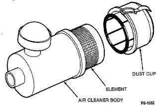
FIGURE 11. TYPICAL AIR CLEANER COMPONENTS
