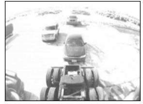
Minimize Blind Spots A real-time rear vision image as seen on the in-cab display unit.
