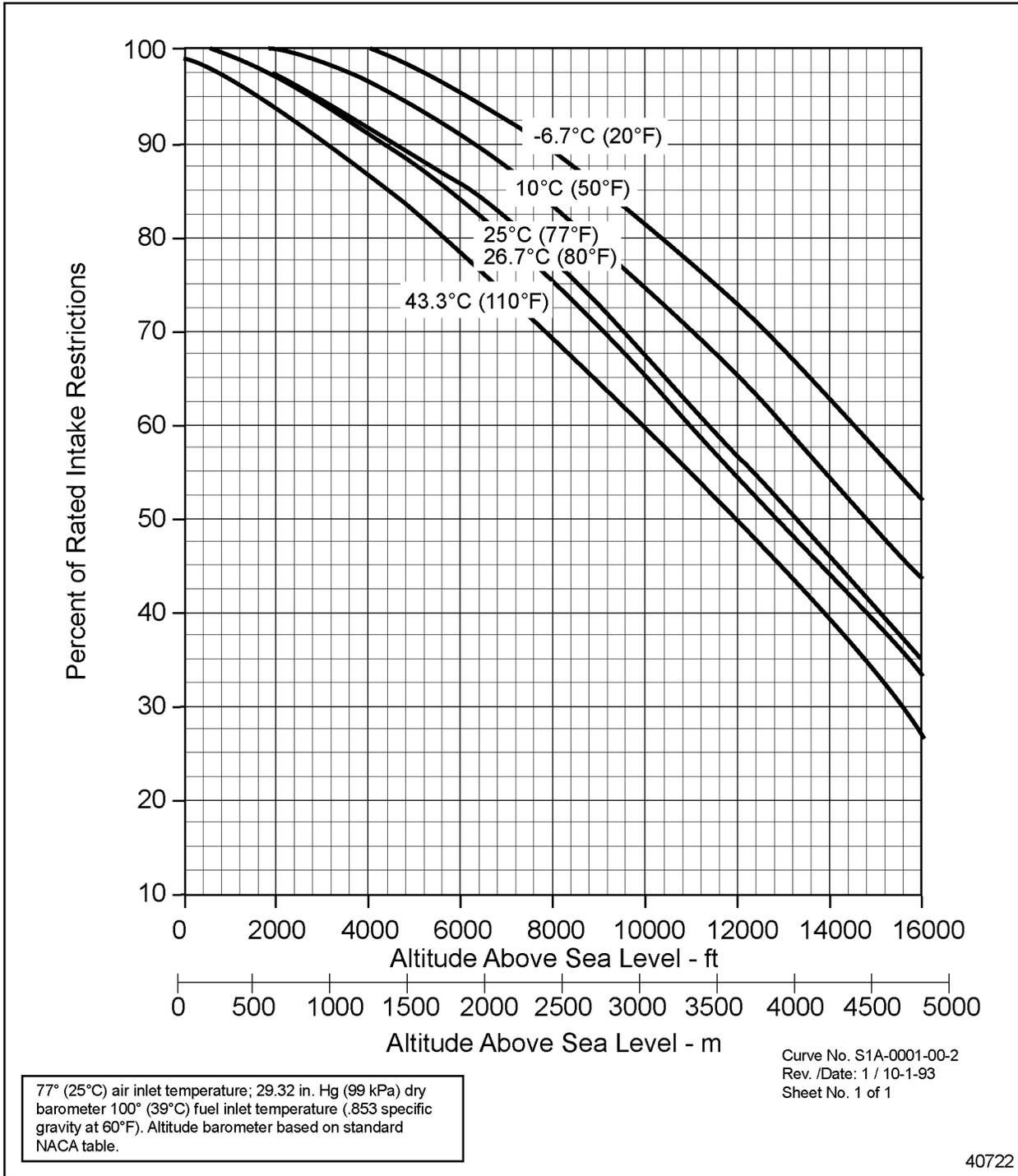
**Figure 4-11 Altitude vs. Inlet Restriction**
