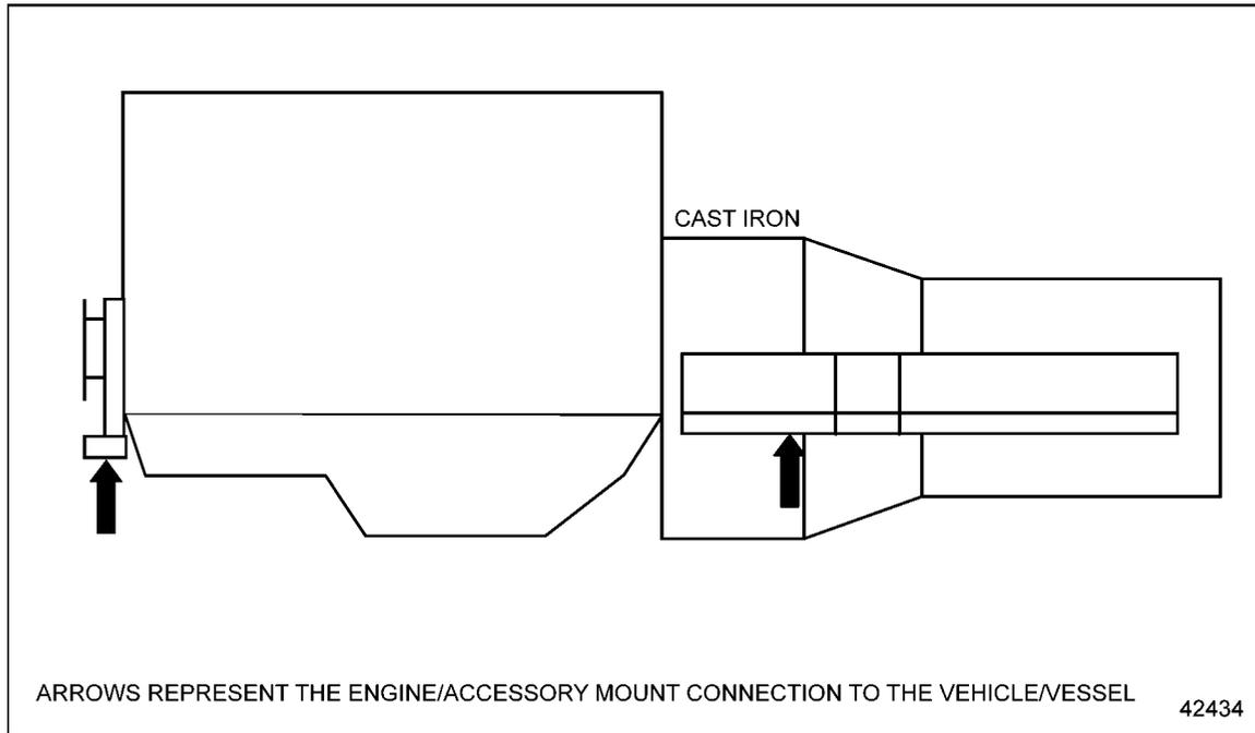
**Figure 12-2 Three-Point Mounting with a Set of Rear Cradle Mounts**
