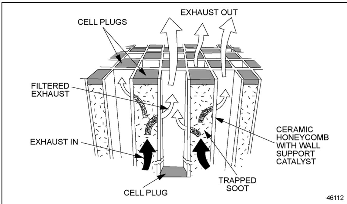
**Figure 7-5 Operation of the Diesel Particulate Filter**
