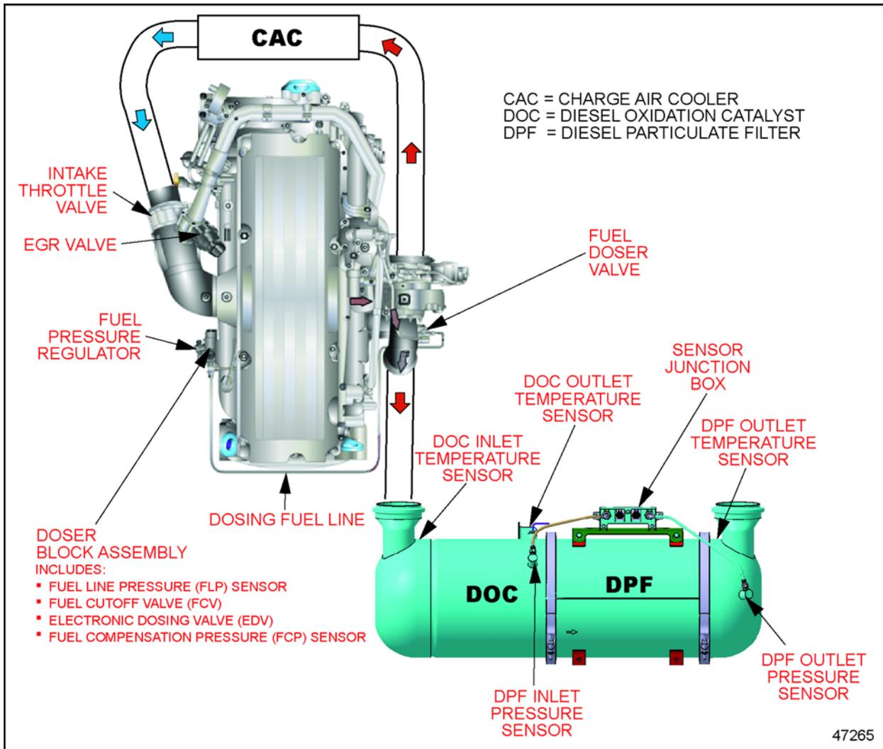
Figure 7-2 Series 60 Aftertreatment System Schematic
