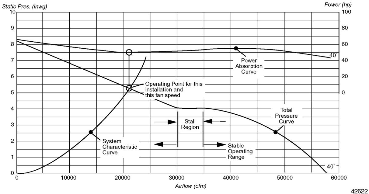
Figure 8-18 Typical Fan Performance Curve
