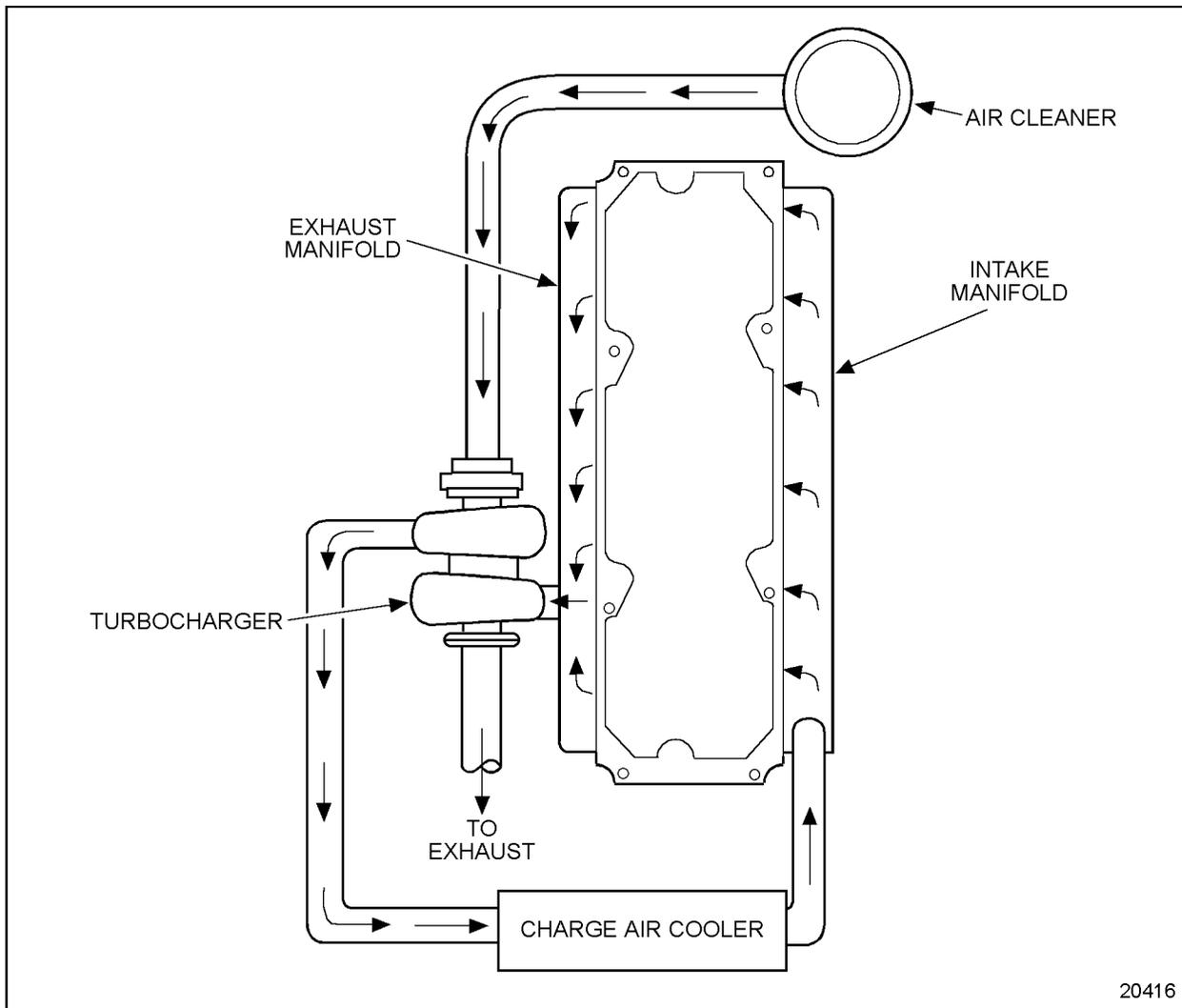
**Figure 4-1 Air Intake System Schematic – On-Highway**
