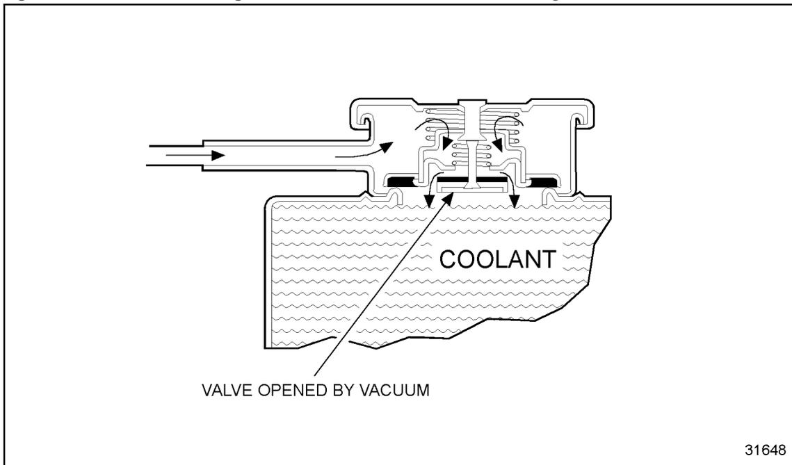
**Figure 8-27 Pressure Control Cap — Vacuum Valve Open**
