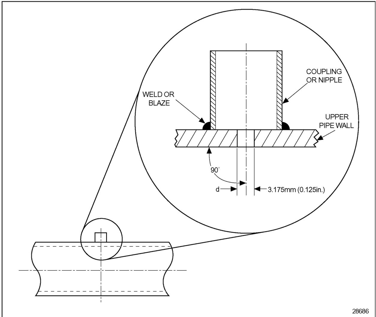
Figure 8-42 Static Pressure Tap
