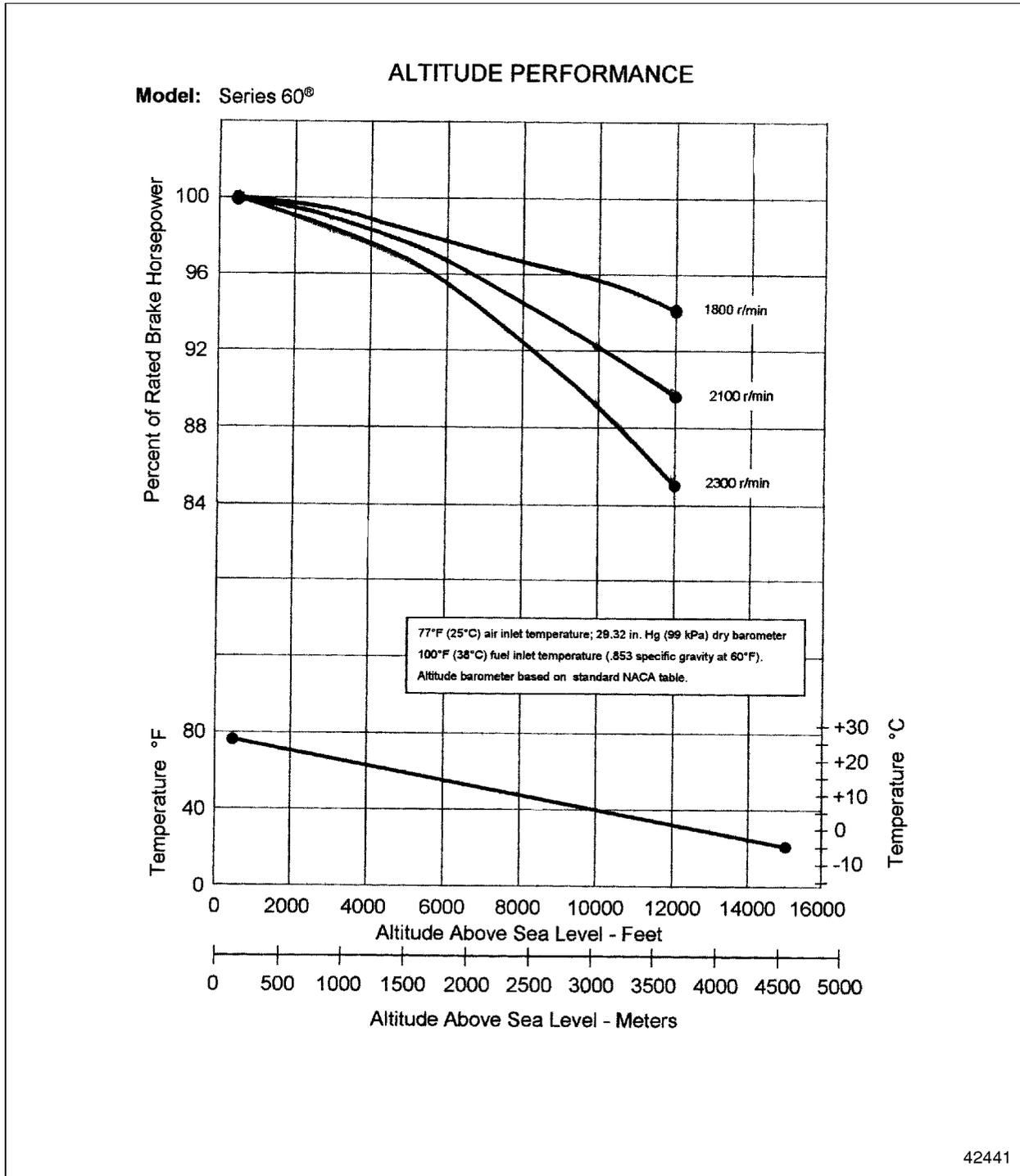
**Figure 15-3 The Effects Of Altitude On Engine Power**
