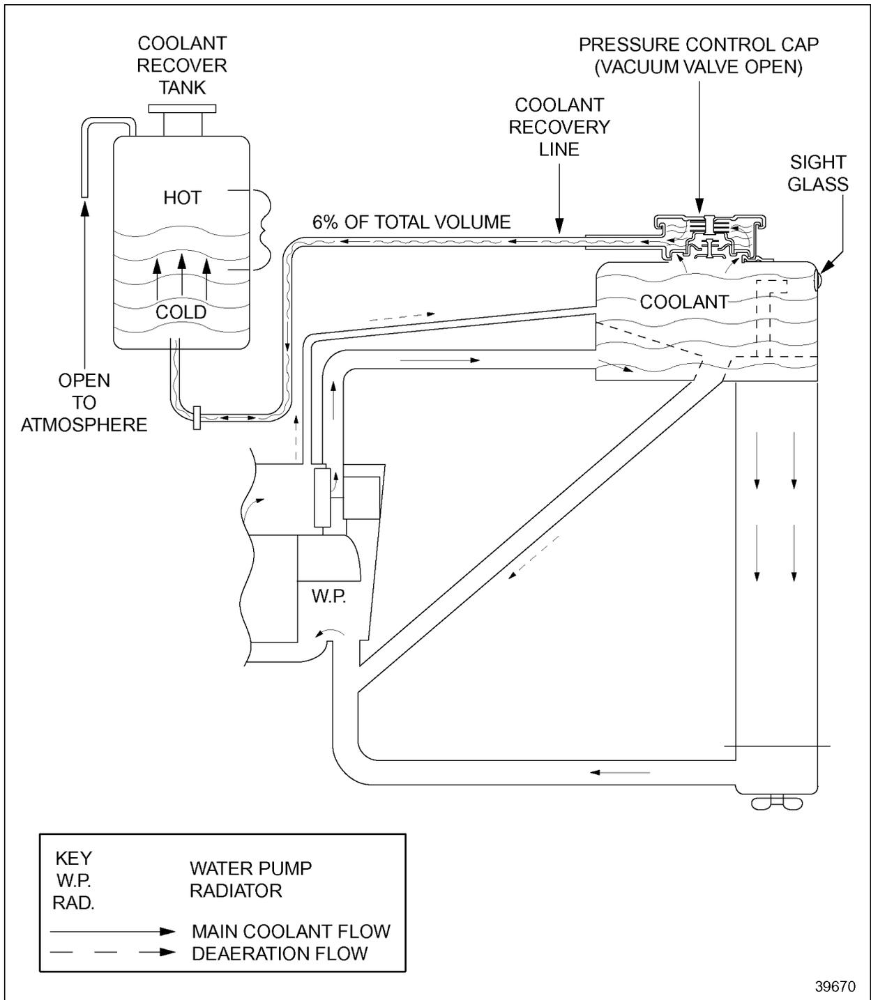
**Figure 8-32 Cooling System Design (Stabilized Temperature — Open Thermostat)**
