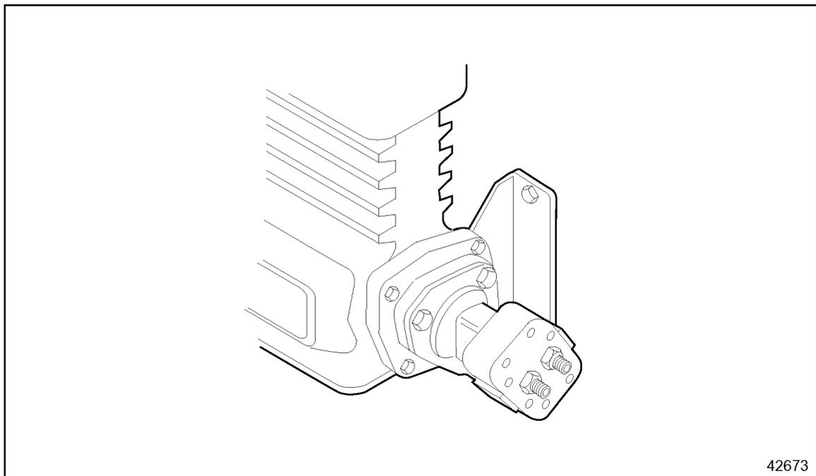
**Figure 16-2 Air Compressor Mounted Fuel Pump**
