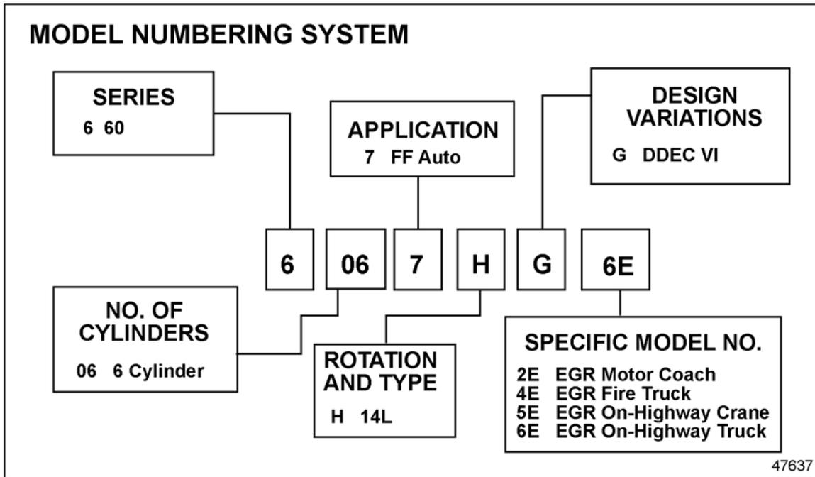
Figure 3-7 Detroit Diesel Engine Model Numbering System — On-Highway
