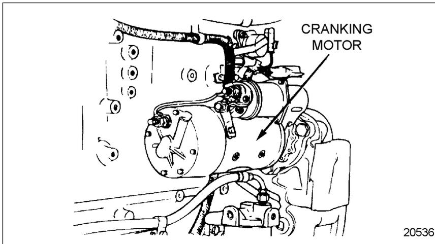
**Figure 11-3 Cranking Motor Mounting**
