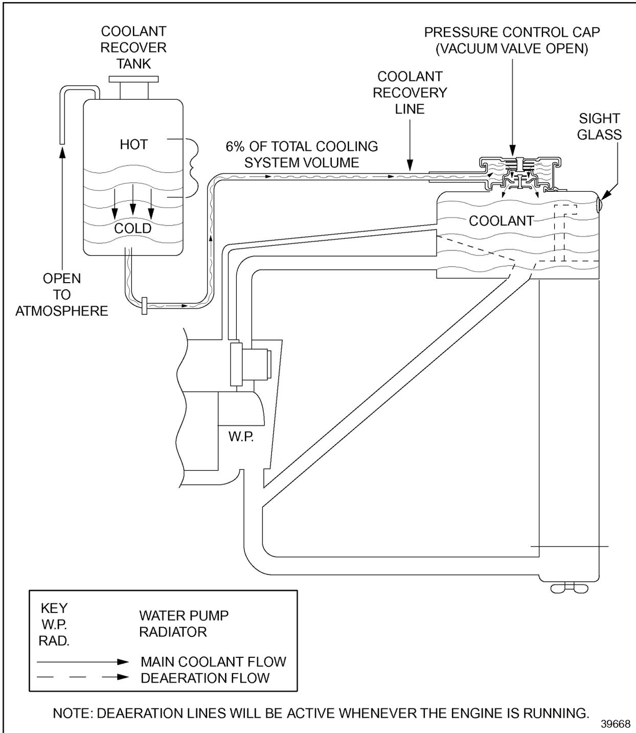
**Figure 8-33 Cooling System Design (Cool-down — Closed Thermostat)**
