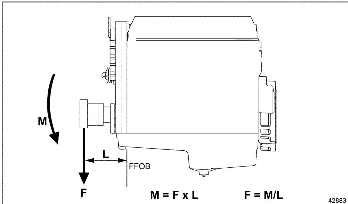
**Figure 17-2 Bending Moment on the Front of the Crankshaft**
