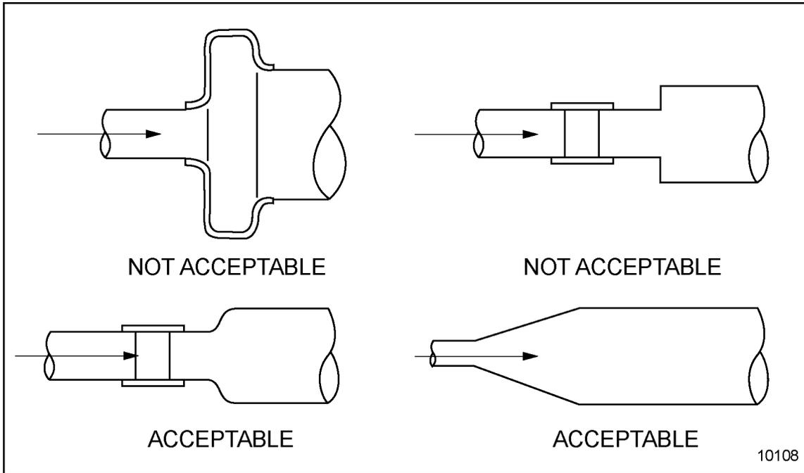
**Figure 4-12 Diffuser Configurations**
