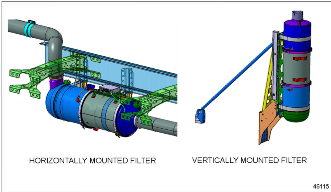
**Figure 7-10** Typical Mounting Views of an Aftertreatment Device
