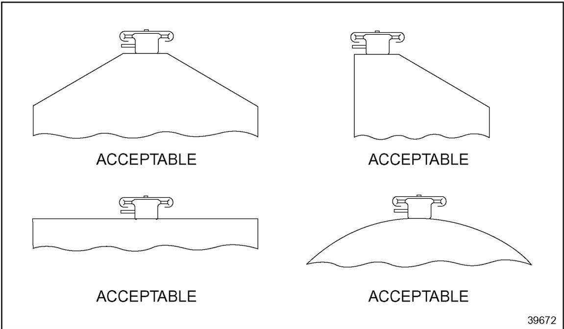
**Figure 8-34 Acceptable Top Tank Design**
