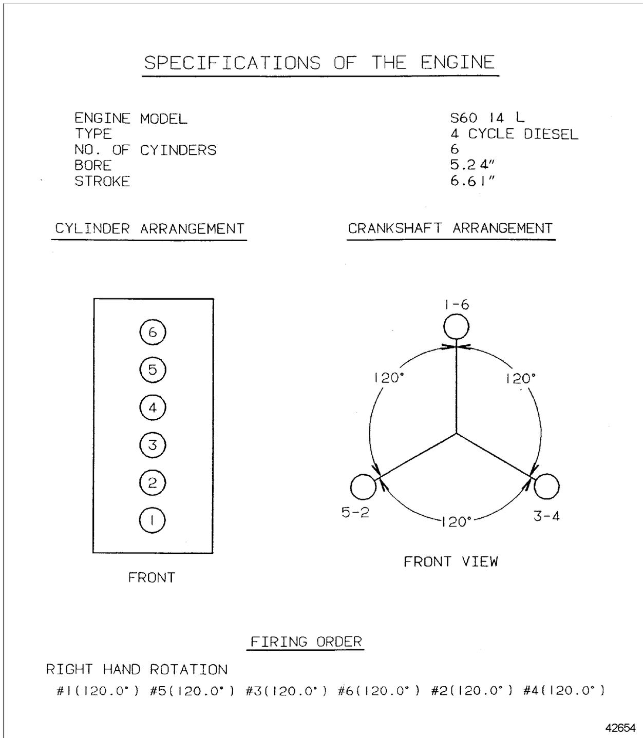
**Figure 13-1 Engine Specifications of the Series 60 14 L Engine**
