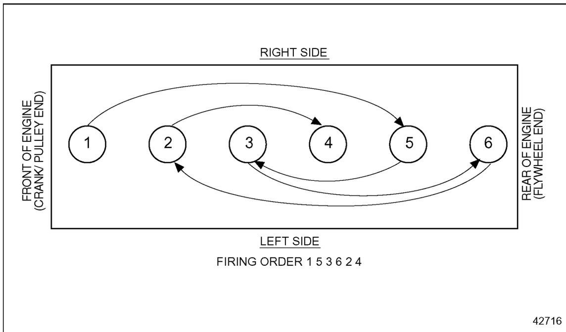
**Figure 3-3**      **Cylinder Designation and Firing Order, Series 60**
