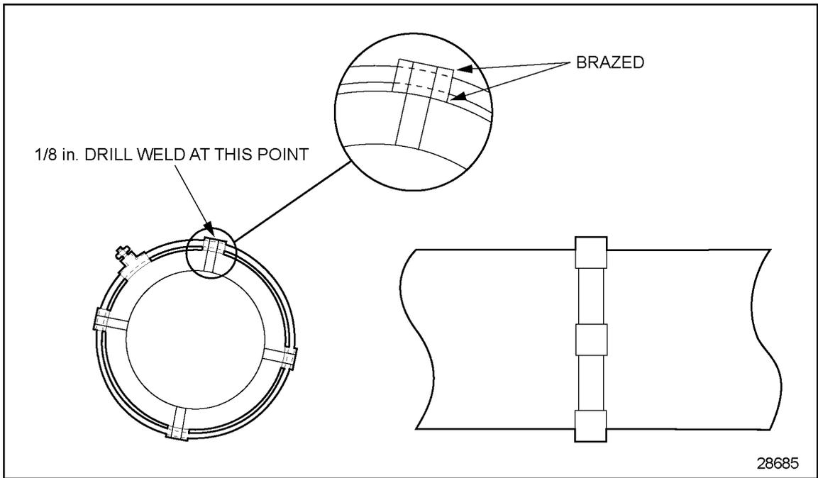
**Figure 6-7 Piezometer Ring**
