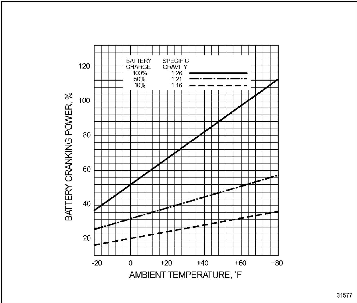
Figure 18-2 Battery Cranking Power - Percent
