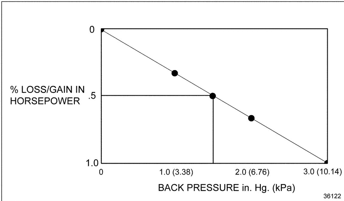
**Figure 15-2 The Effects of Exhaust Back Pressure on Engine Power**
