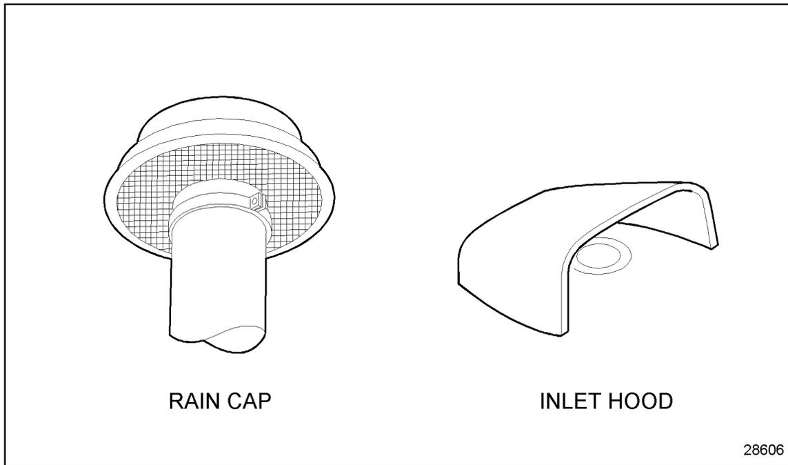
**Figure 4-10 Rain Cap and Inlet Hood**
