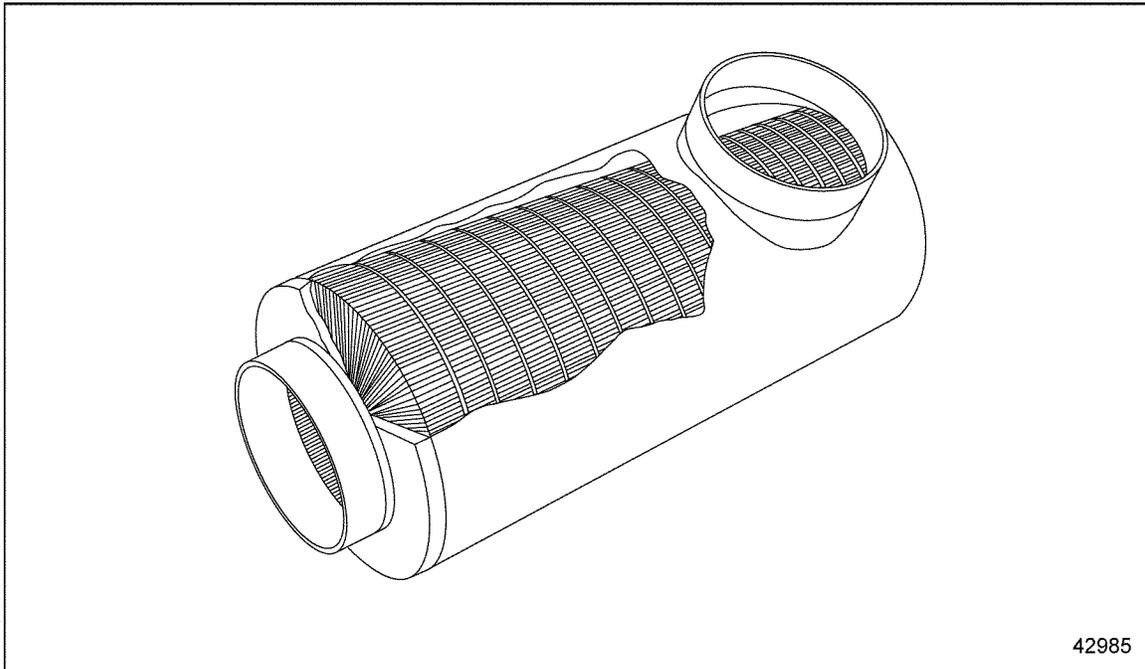
**Figure 4-5** Light-Duty Air Cleaner, Single Stage Cartridge Type
