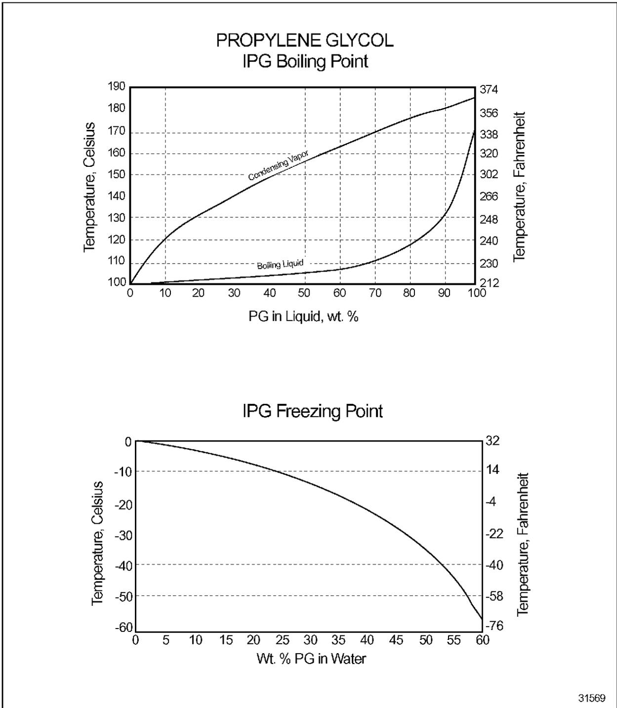
**Figure 18-1 Coolant Freezing and Boiling Temperature vs. Inhibited Propylene Glycol (IPG) Concentration (Sea Level)**
