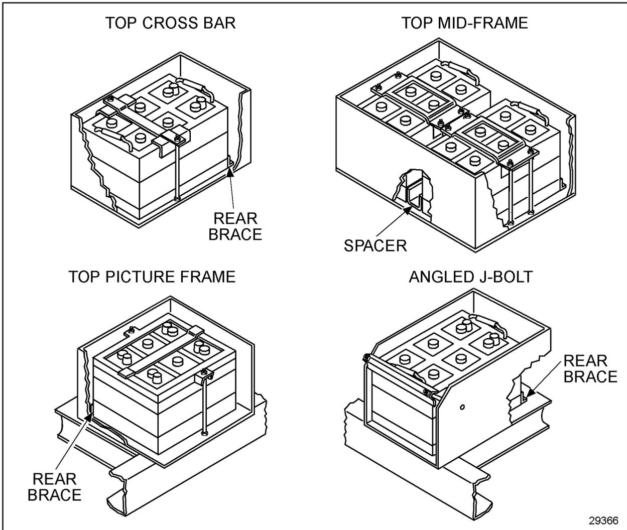
Figure 11-2 Battery Retainers
