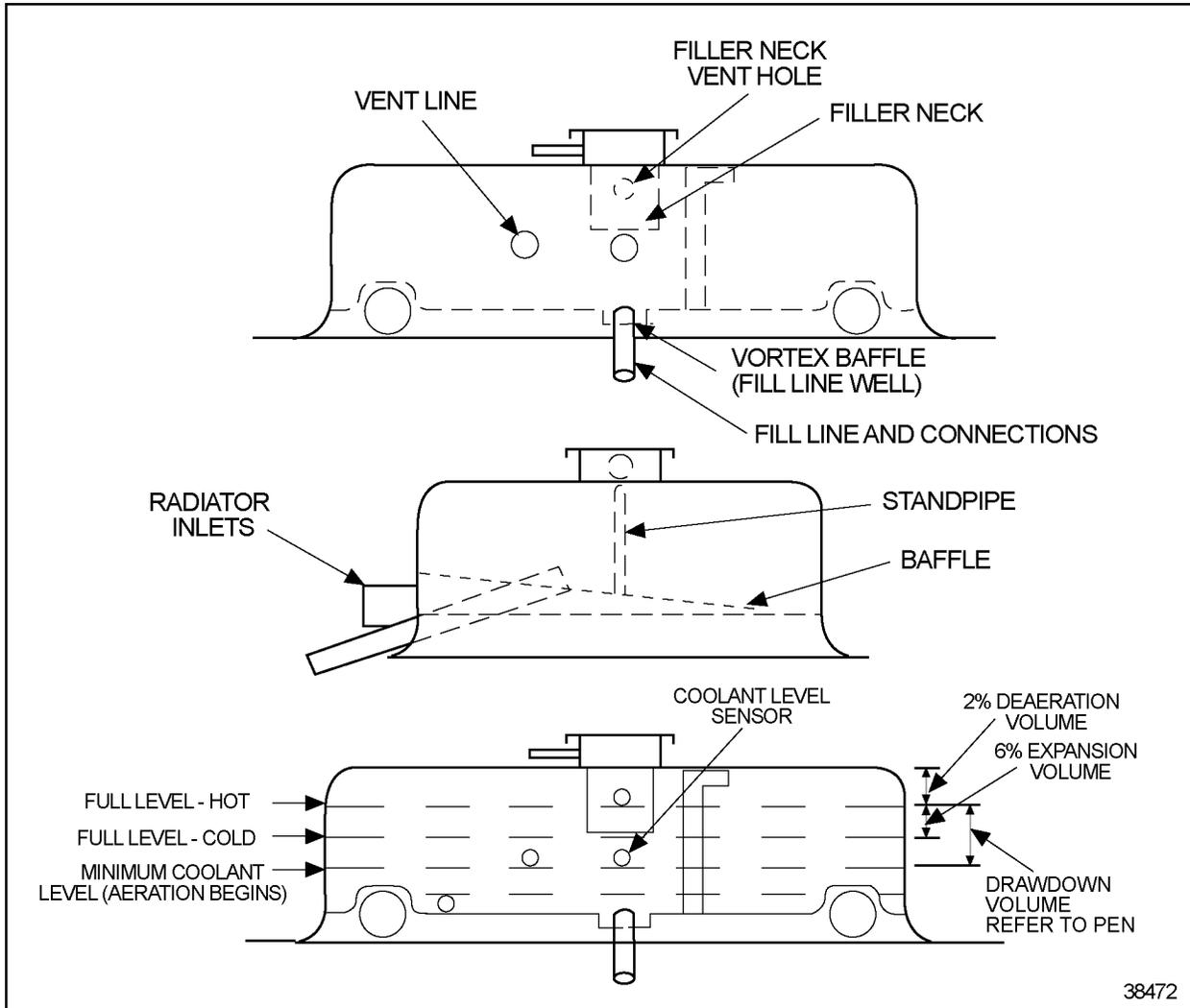
**Figure 8-21 Rapid Warm-up Down Flow Radiator Top Tank**
