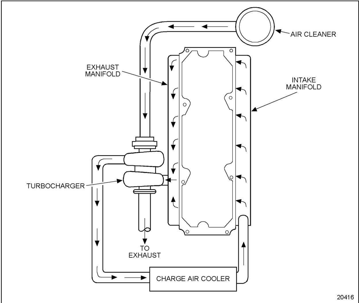
**Figure 6-1 Exhaust System Schematic**
