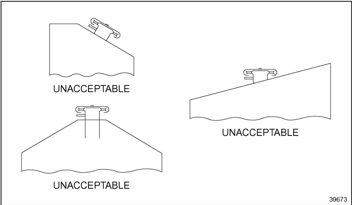
**Figure 8-35 Unacceptable Top Tank Design**
