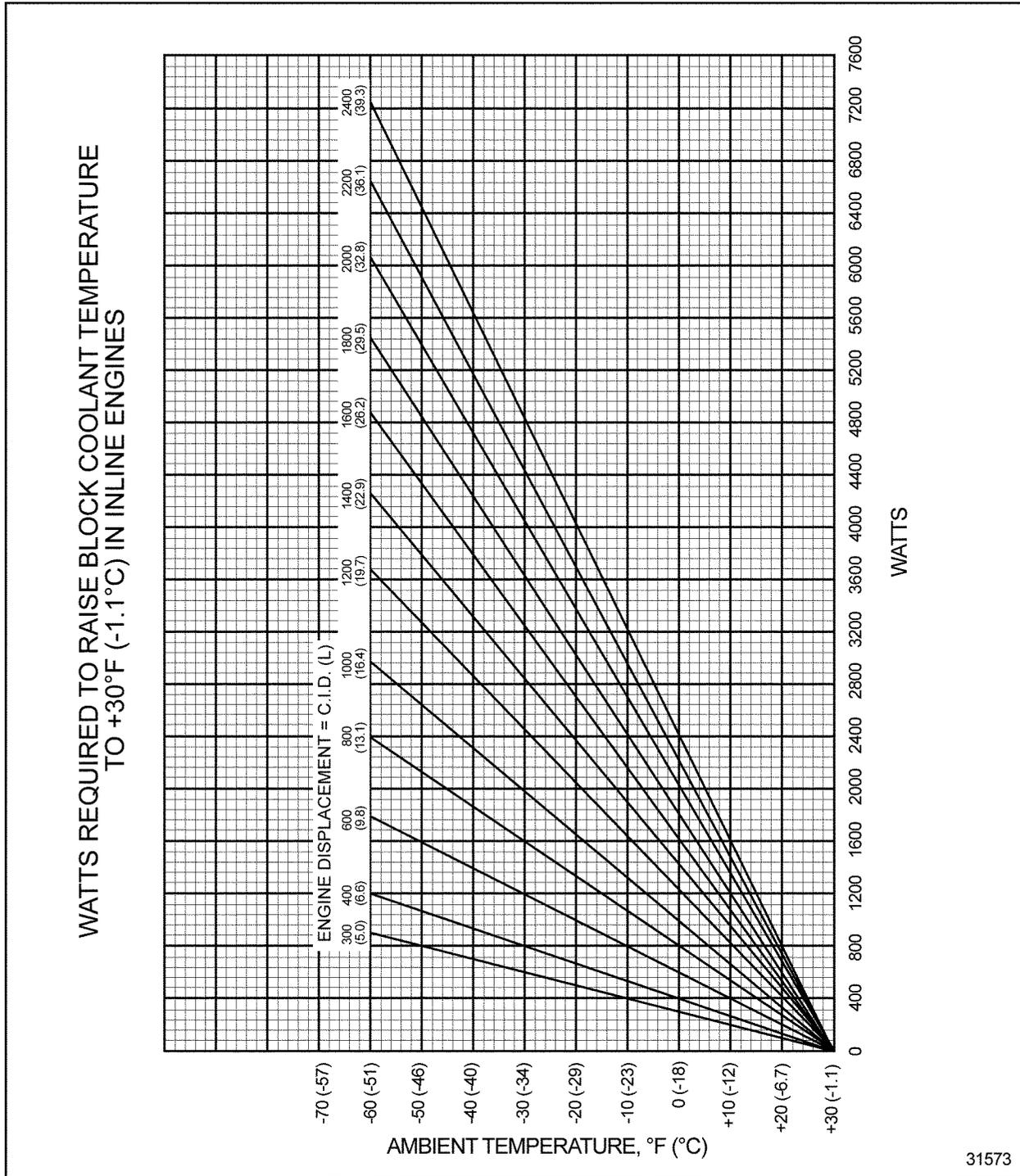
**Figure 18-3 Watts Required to Raise Block Coolant Temperature to +30°F (-1.1°C) in Inline Engines**
