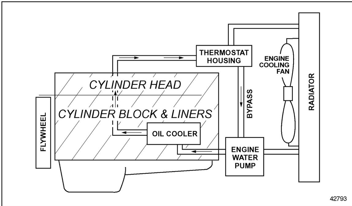
**Figure 8-1 Engine Jacket Water Cooling System — Thermostats Closed**
