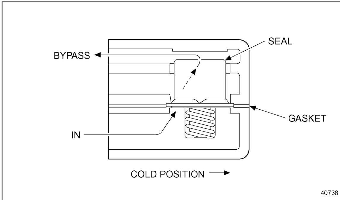
**Figure 8-45** Thermostat Leakage Areas
