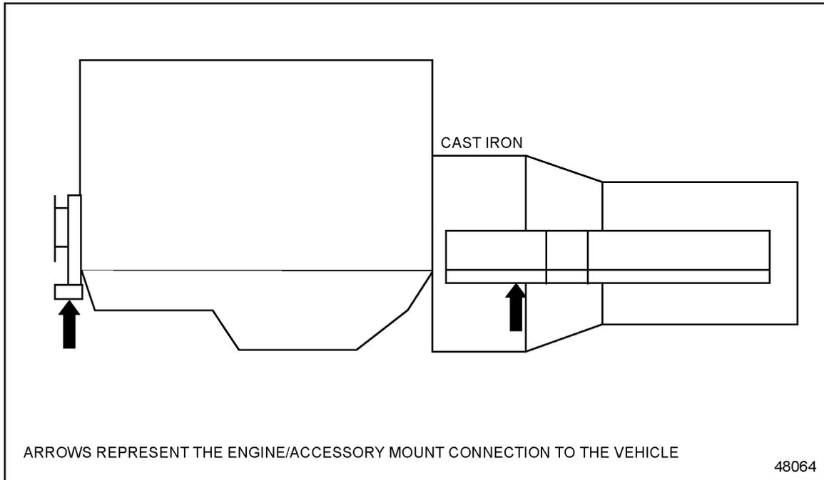
**Figure 12-1 Three Point Mounting with a Set of rear Cradle Mounts**
