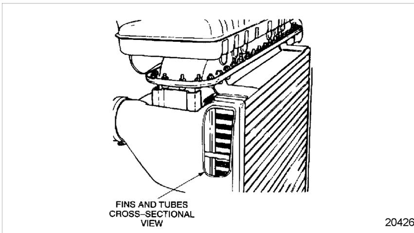
**Figure 8-13 Charge Air Cooler Cross-Section**
