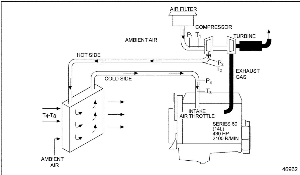
**Figure 4-16 Typical Instrumentation Location**
