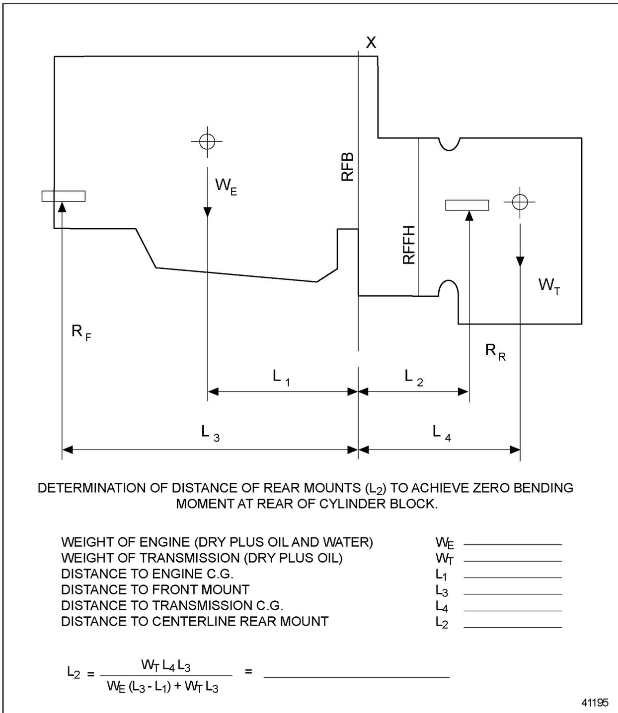
**Figure 12-4 Distance of Rear Mounts for Zero Bending Moments**
