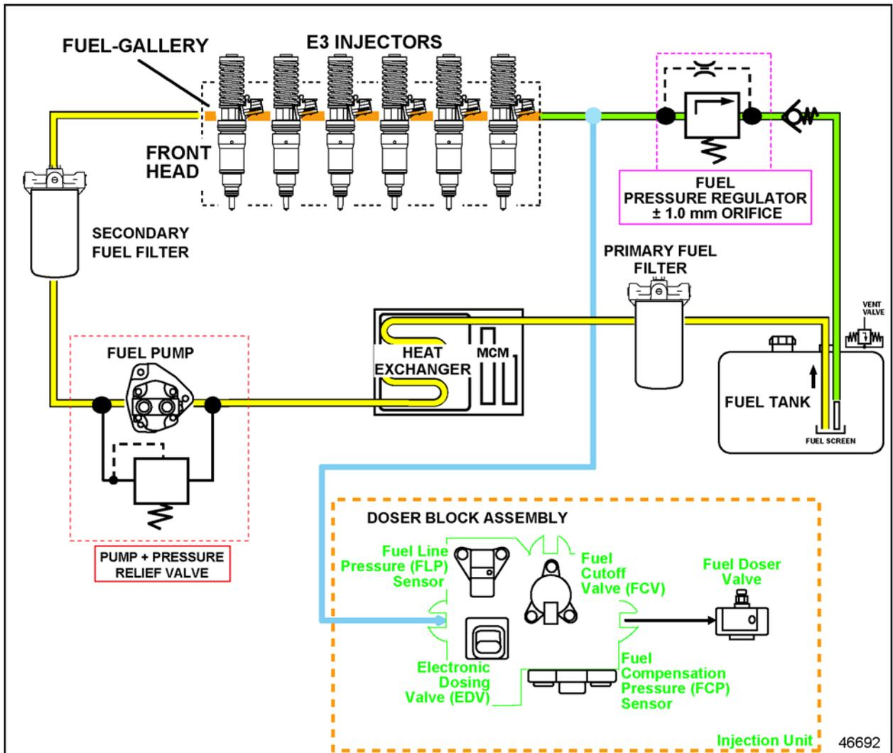
Figure 9-1 Schematic Diagram of the On-Highway Fuel System
