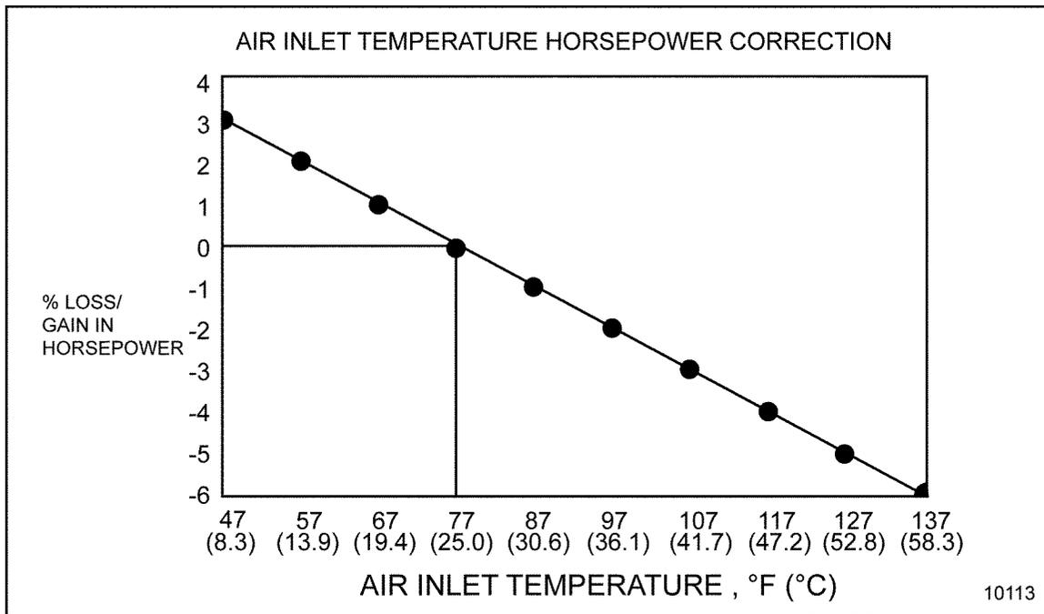
**Figure 15-1 The Effects of Air Inlet Temperature**
