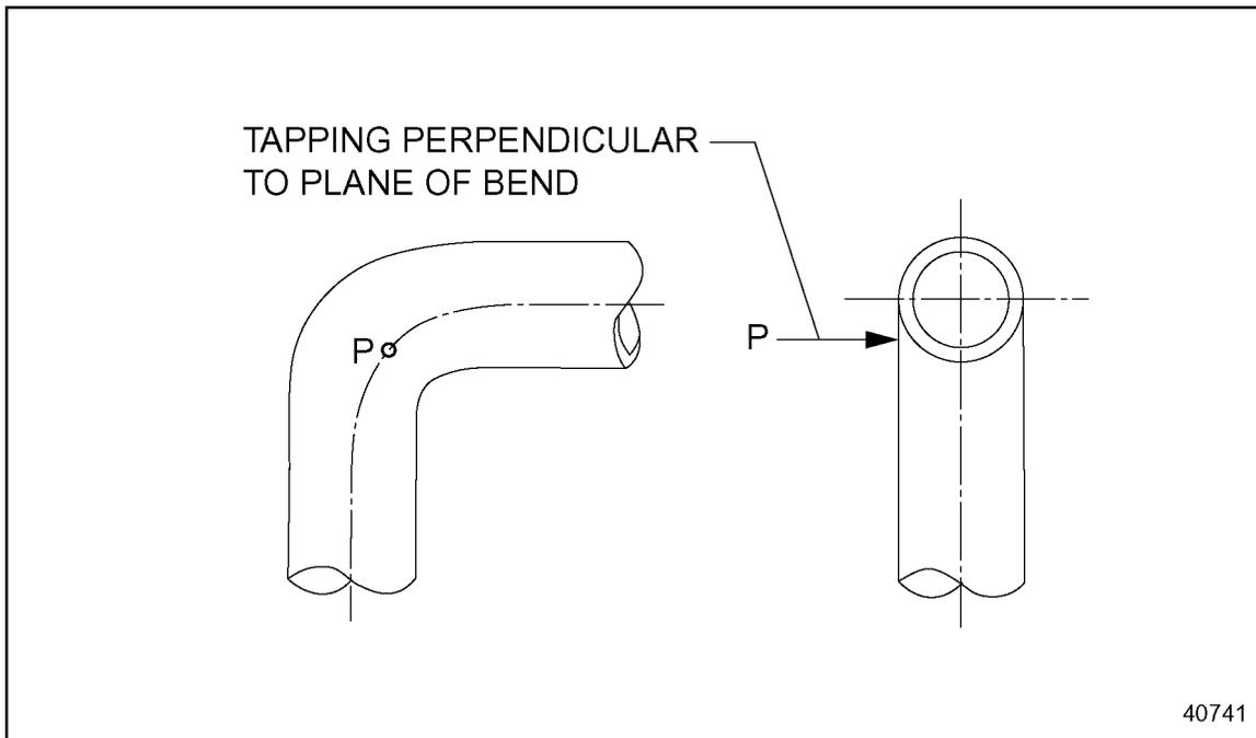
**Figure 8-43**      **Pressure Tap on a Bend**
