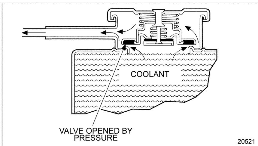
**Figure 8-26 Pressure Control Cap — Pressure Valve Open**
