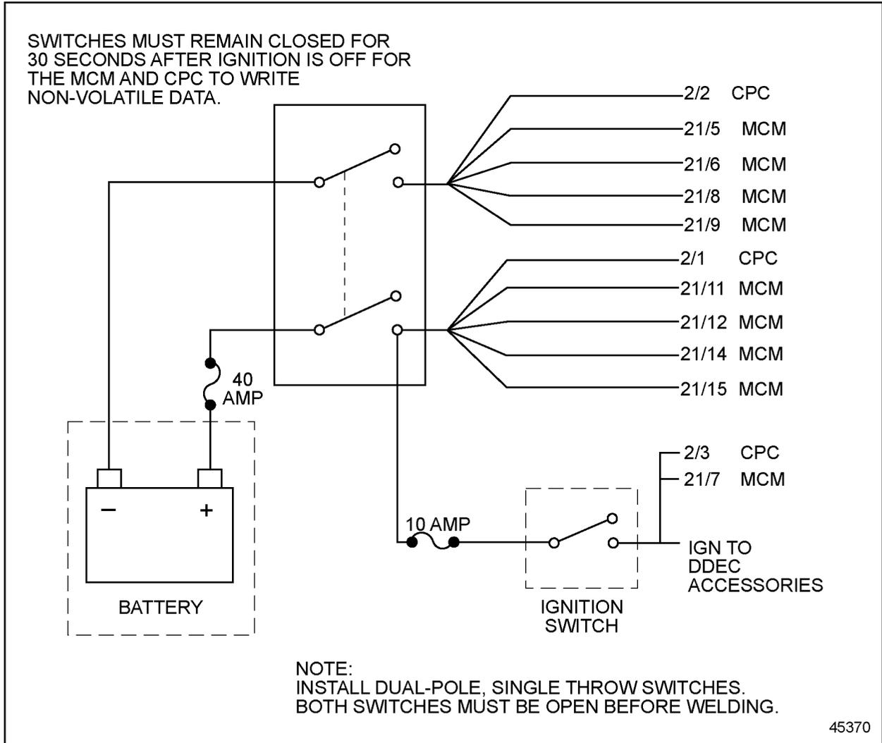
Figure 14-6 Battery Connections for Proper Welding
