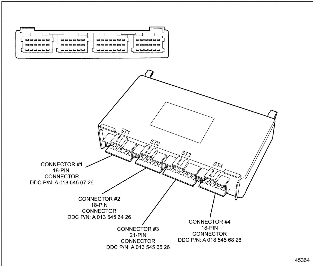
**Figure 14-2 The Common Powertrain Module**
