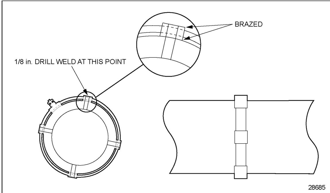
**Figure 8-41** Piezometer Ring
