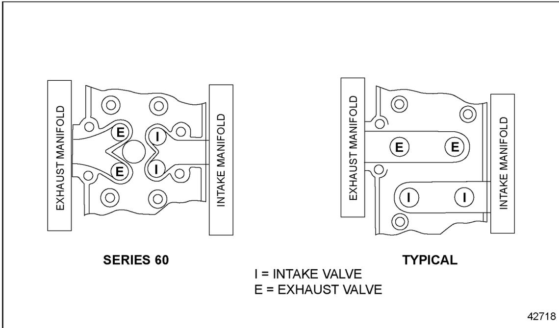
**Figure 3-2 Exhaust and Intake Valves**
