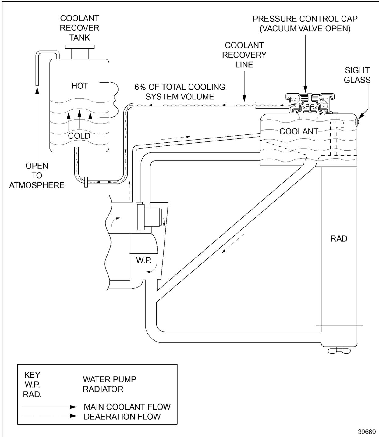
**Figure 8-31 Cooling System Design (Warm-up — Closed Thermostat)**
