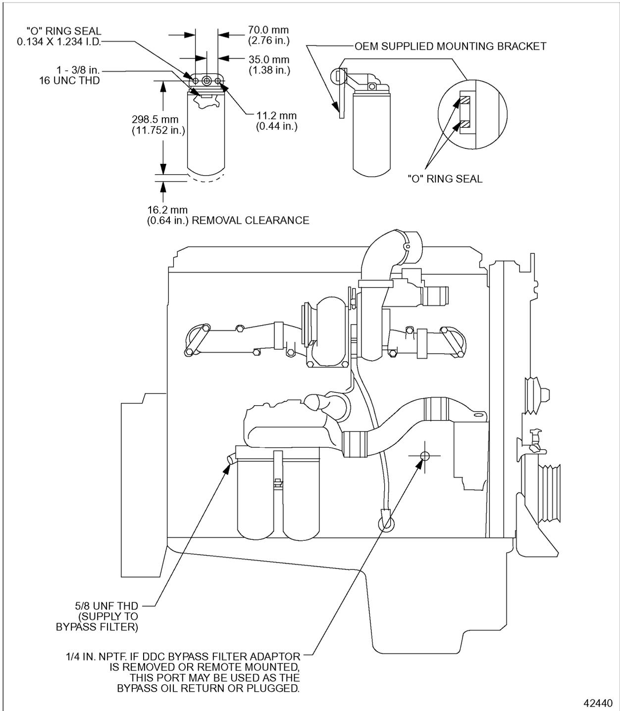
**Figure 10-3 Remote Mount Bypass Filter Options**
