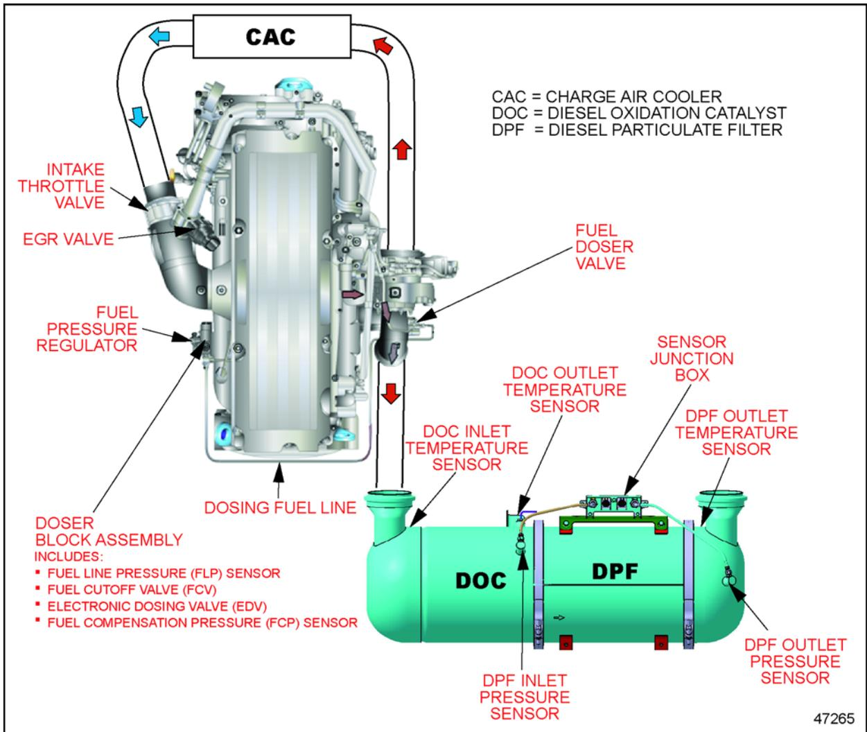
Figure 6-6 Aftertreatment System Schematic
