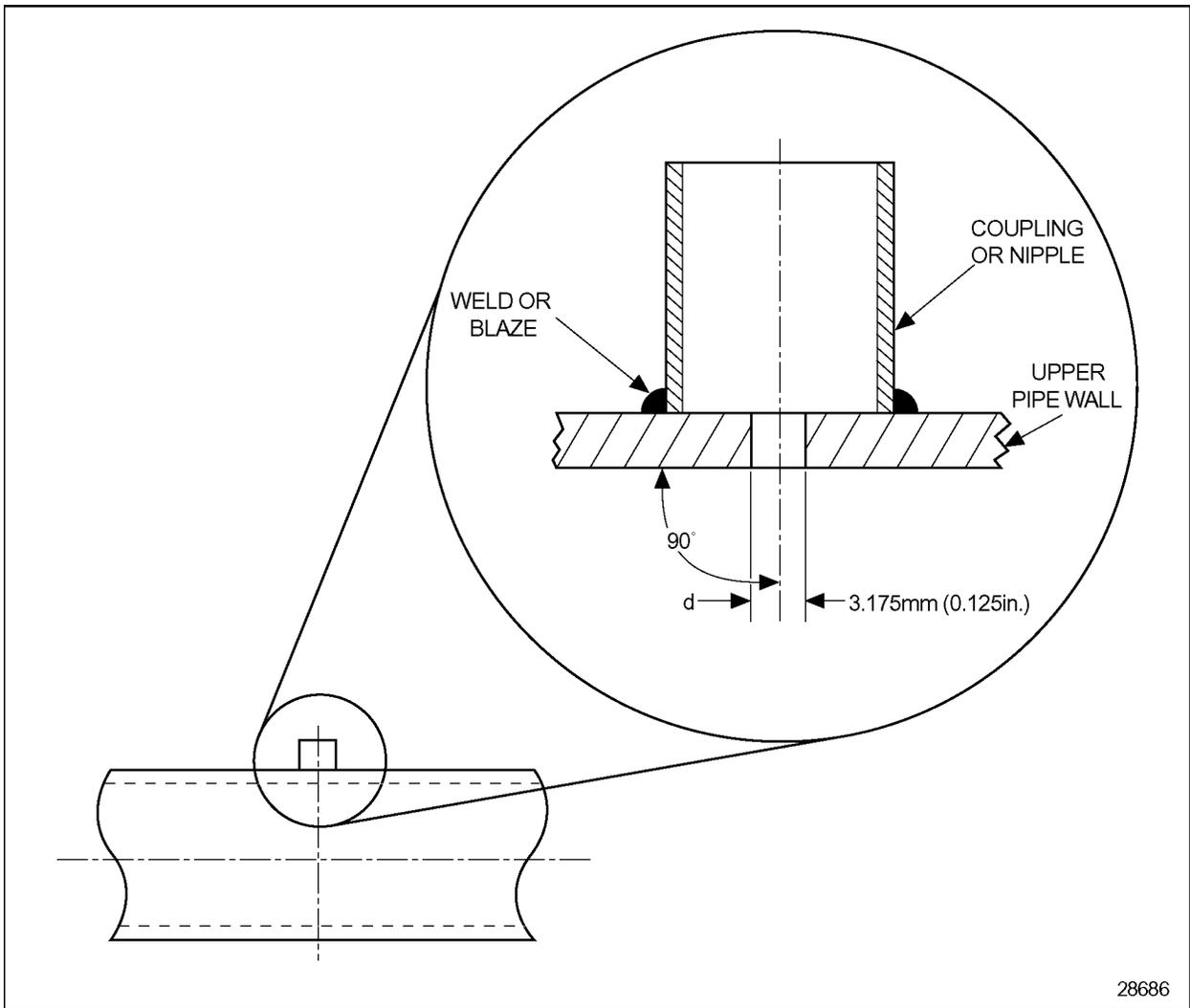
**Figure 6-8 Static Pressure Tap**
