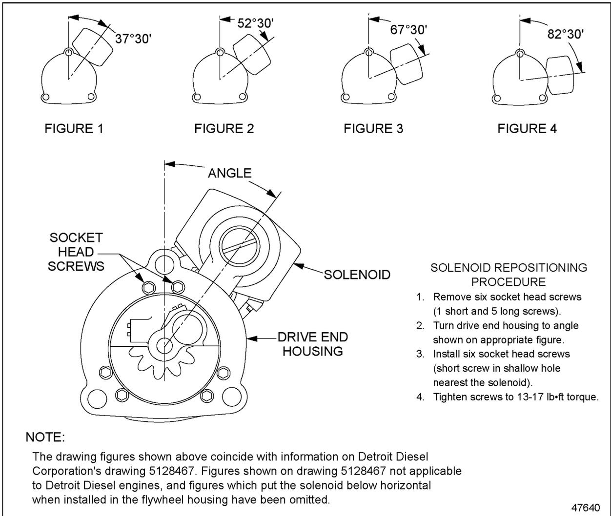
**Figure 11-4      Acceptable Cranking Index with series 60**
