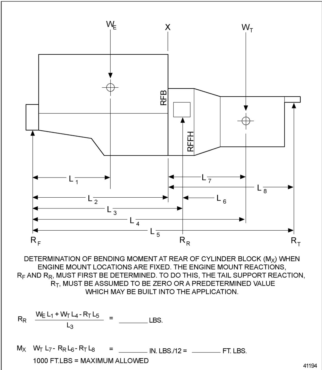
**Figure 12-5 Bending Moment for Fixed Mounting System**
