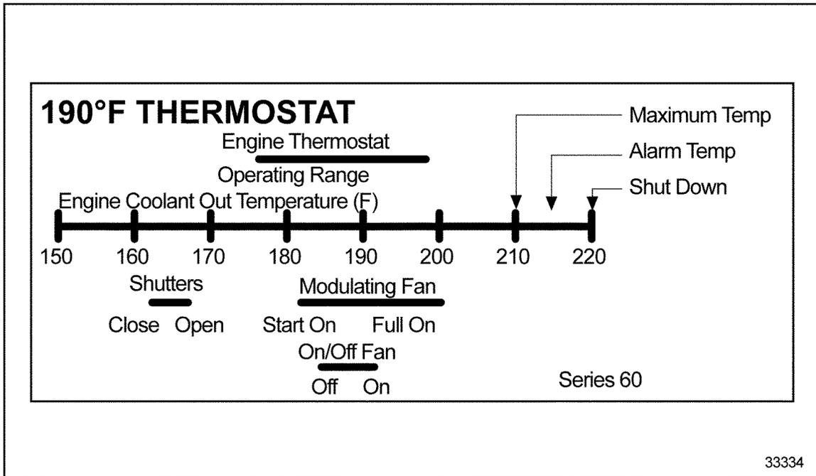
Figure 8-29 Nominal Settings For Coolant Temperature Control Devices — 190°
