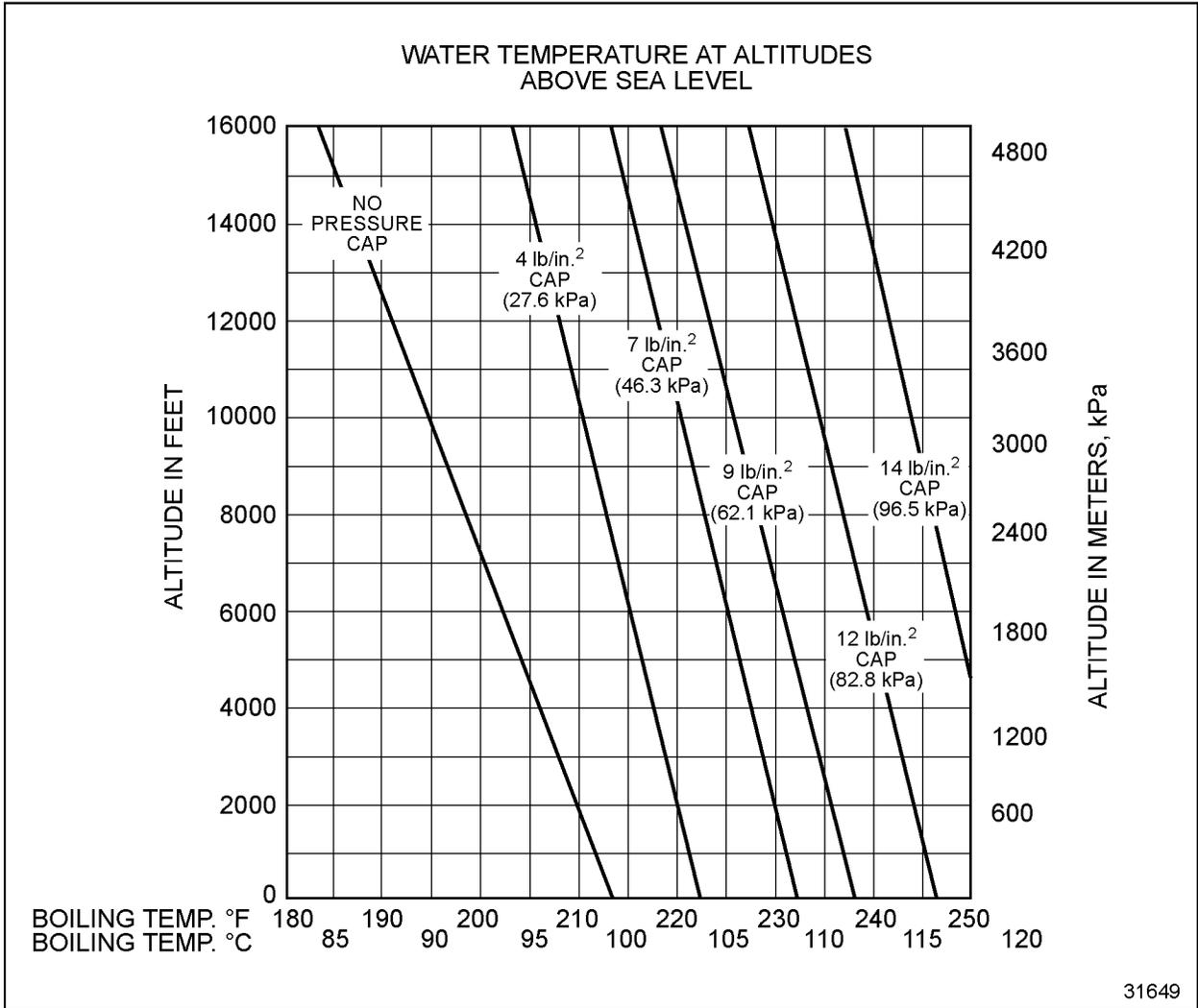
**Figure 8-28 Effect of Altitude and Pressure Caps**
