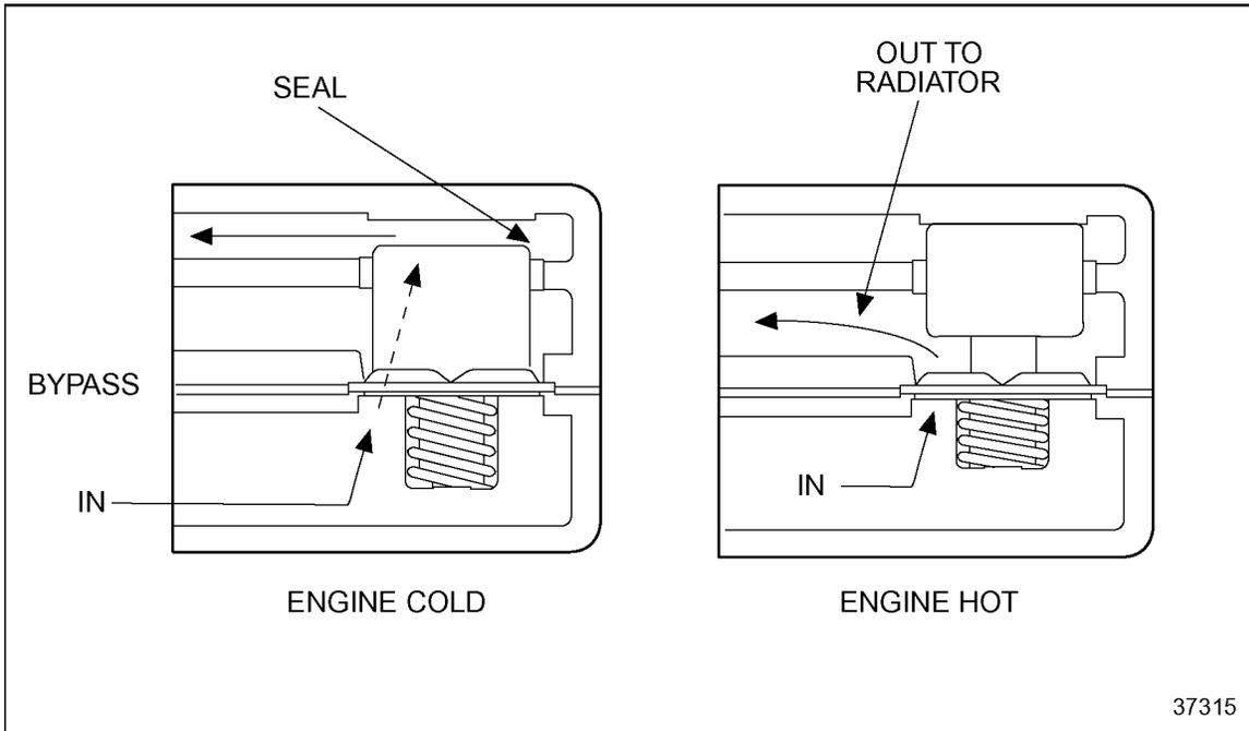
**Figure 8-36 Full Blocking Thermostat (Top Bypass)**
