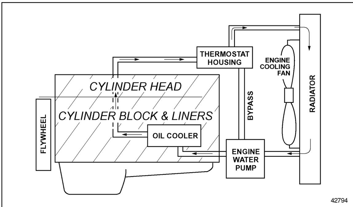
**Figure 8-2 Engine Jacket Water Cooling System — Thermostats Fully Open**
