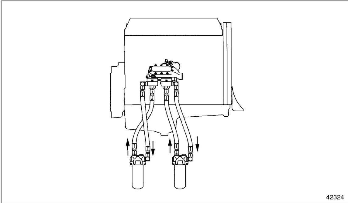
**Figure 10-2** Typical Hose Routing for Remote-mounted Filter Adapters
