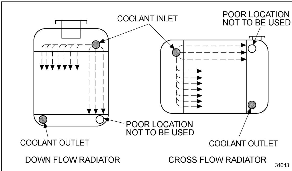
**Figure 8-20 Down Flow Radiator and Cross Flow Radiator**
