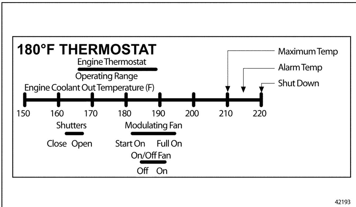
Figure 8-30 Nominal Settings For Coolant Temperature Control Devices — 180°
