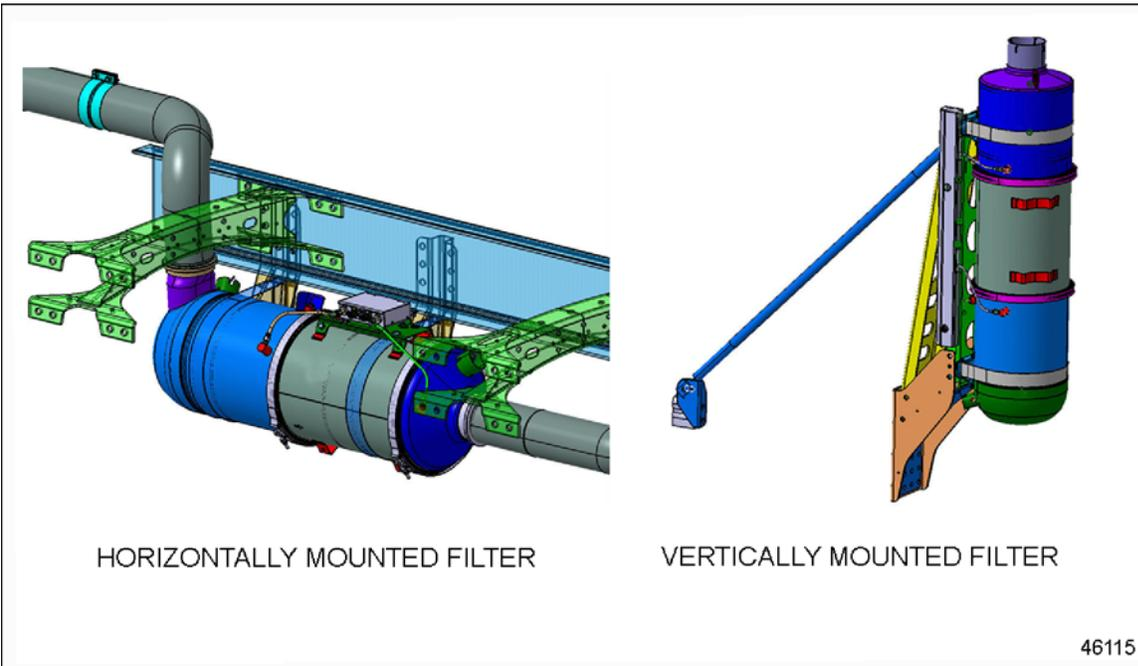
**Figure 7-13 Aftertreatment Device Orientation Variations**
