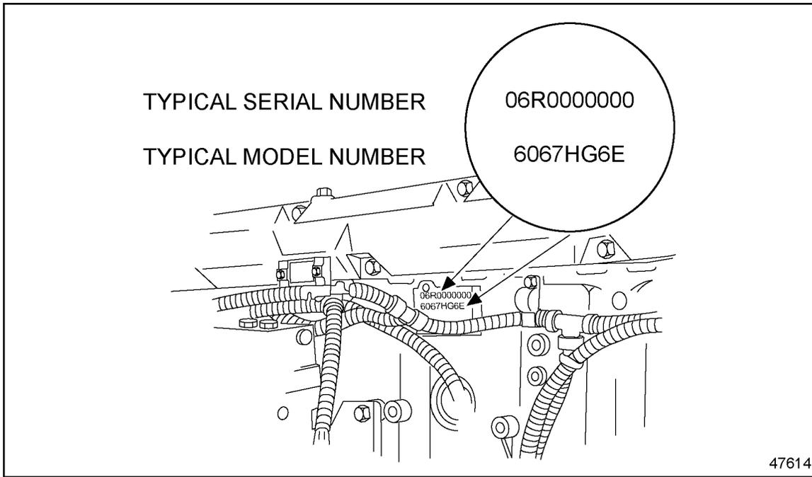
**Figure 3-6 The Engine Serial Numbers Stamp and Model Number, Series 60**
