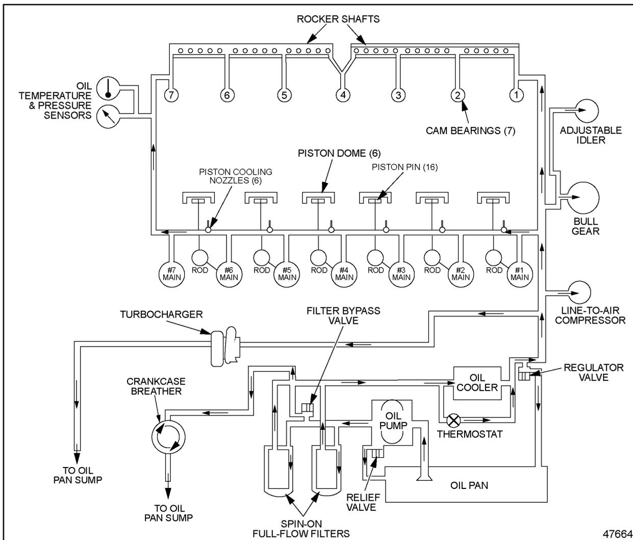
**Figure 10-1 Schematic Diagram of Current Lubrication System**
