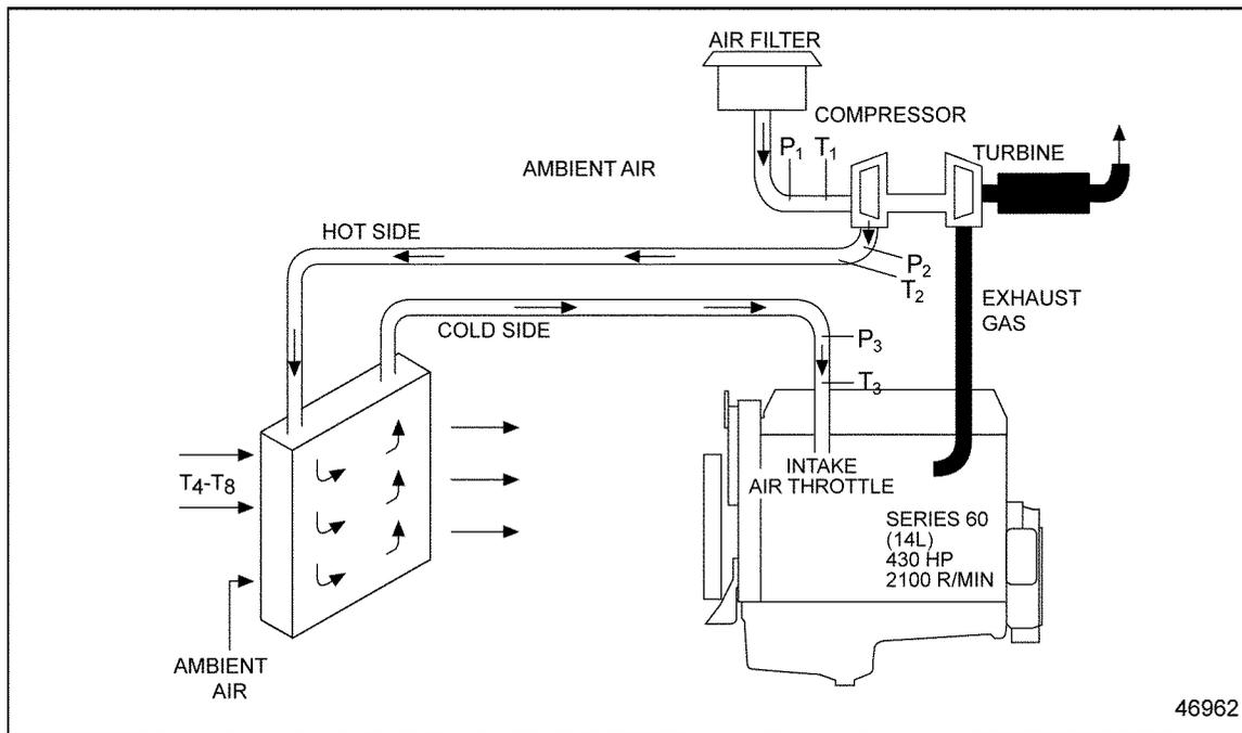
**Figure 8-44 Typical Instrumentation Location**
