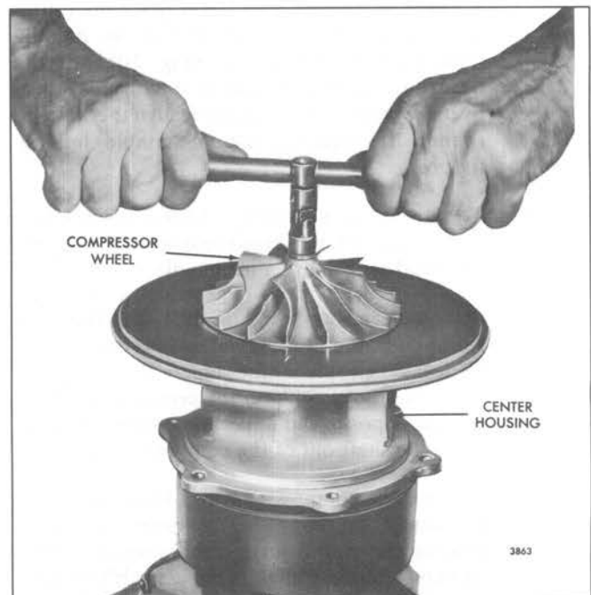
Fig. 14 – Tightening Compressor Wheel Lock Nut using Holding Fixture J 21225
