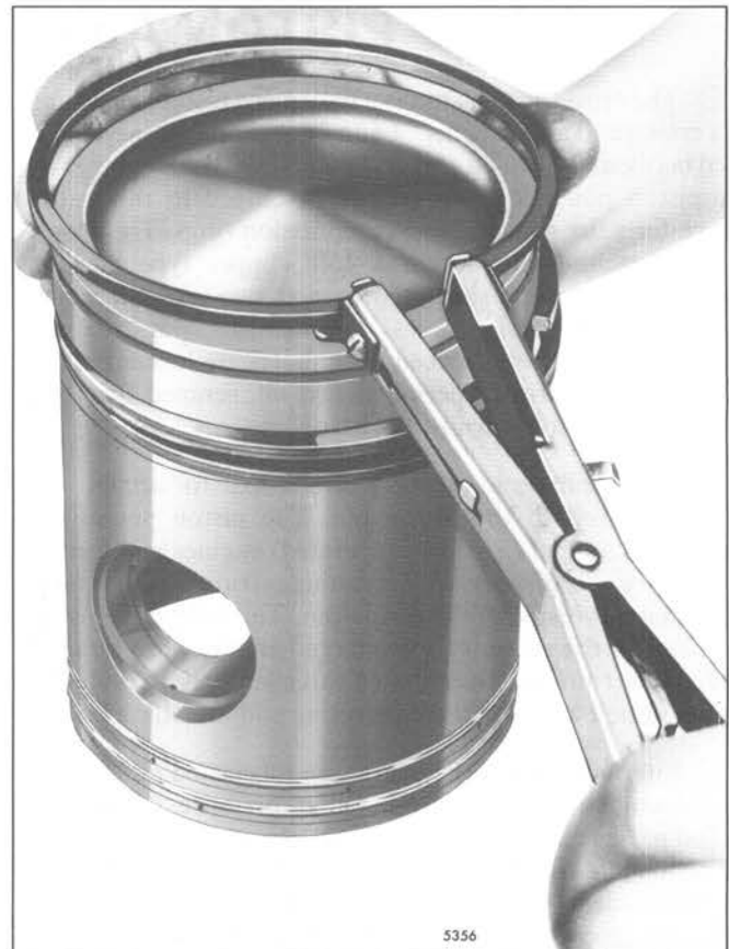
Fig. 5 - Removing or Installing Piston Rings using Tool J 8128
