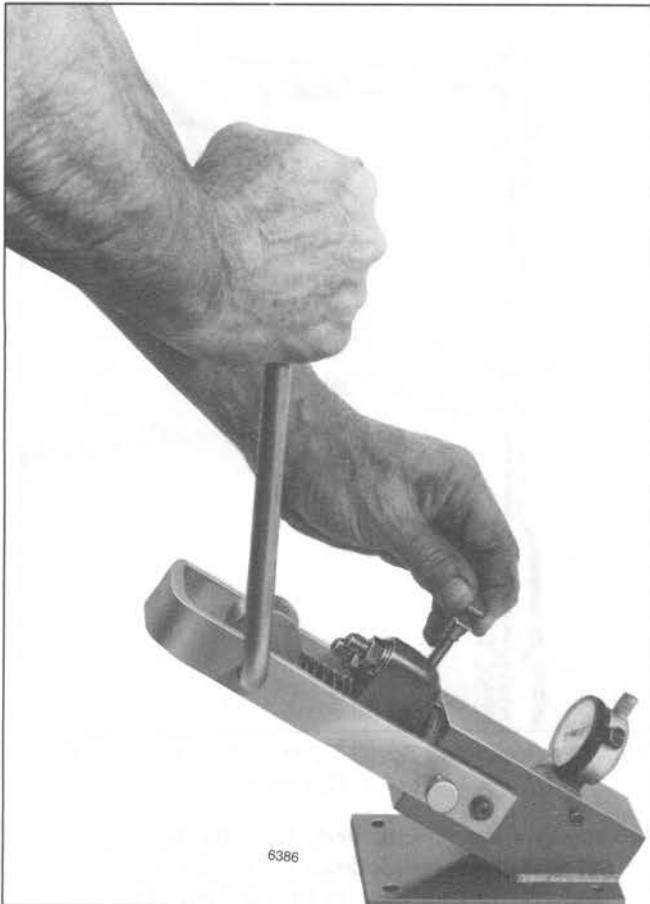
Fig. 7 – Checking Rack for Freeness in Tester J 29584
