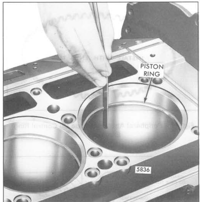
Fig. 15 - Measuring Piston Ring Gap
