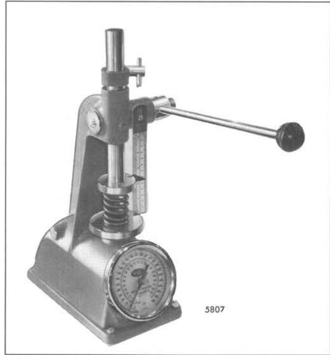
Fig. 6 - Testing Cam Follower Spring with Tool J 22738-02
