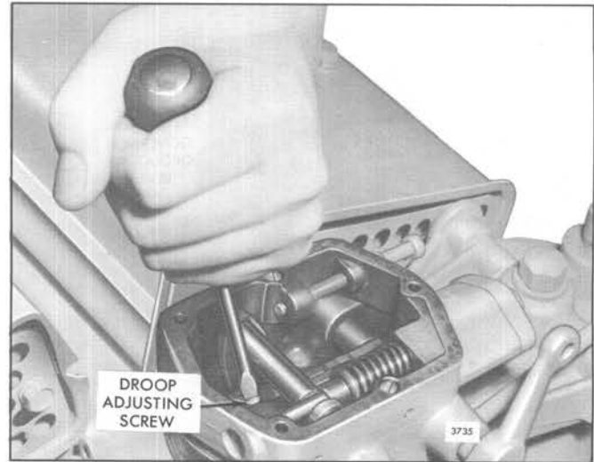
Fig. 10 – Adjusting Speed Droop
