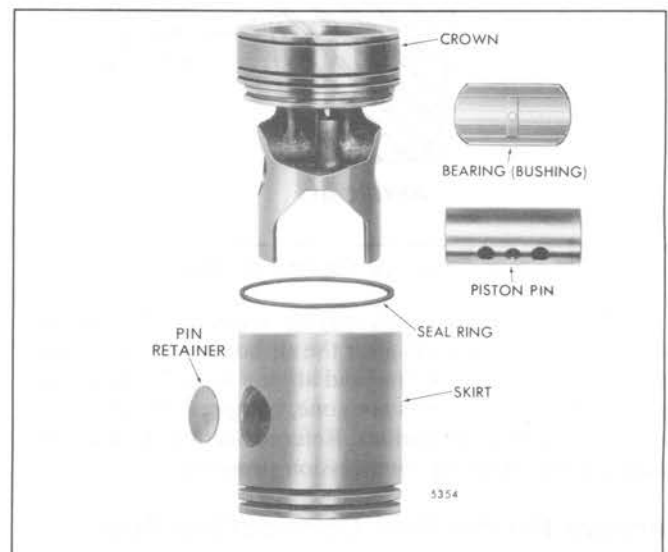
Fig. 2 - Cross-Head Piston and Connecting Rod Components
