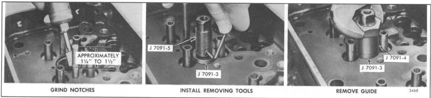
Fig. 8 – Removing Press-Fit Exhaust Valve Bridge Guide
