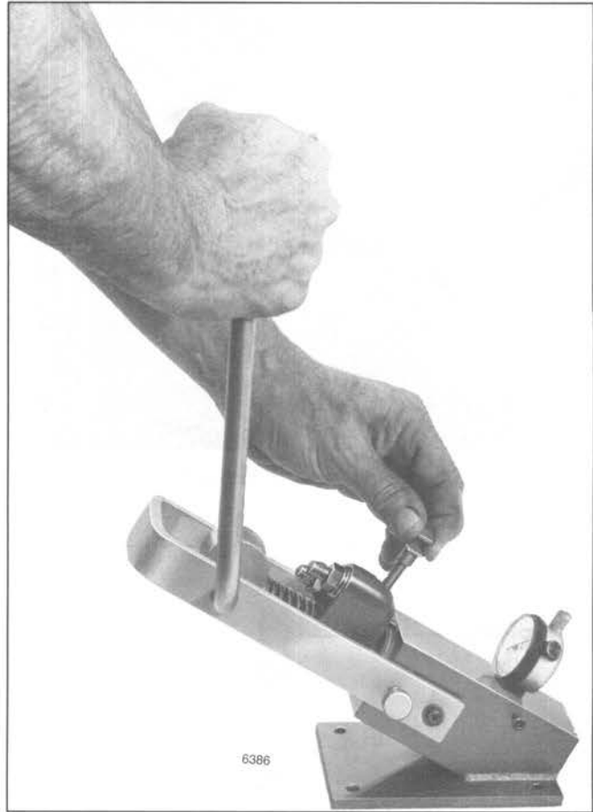
Fig. 36 – Checking Rack for Freeness in Tester J 29584
