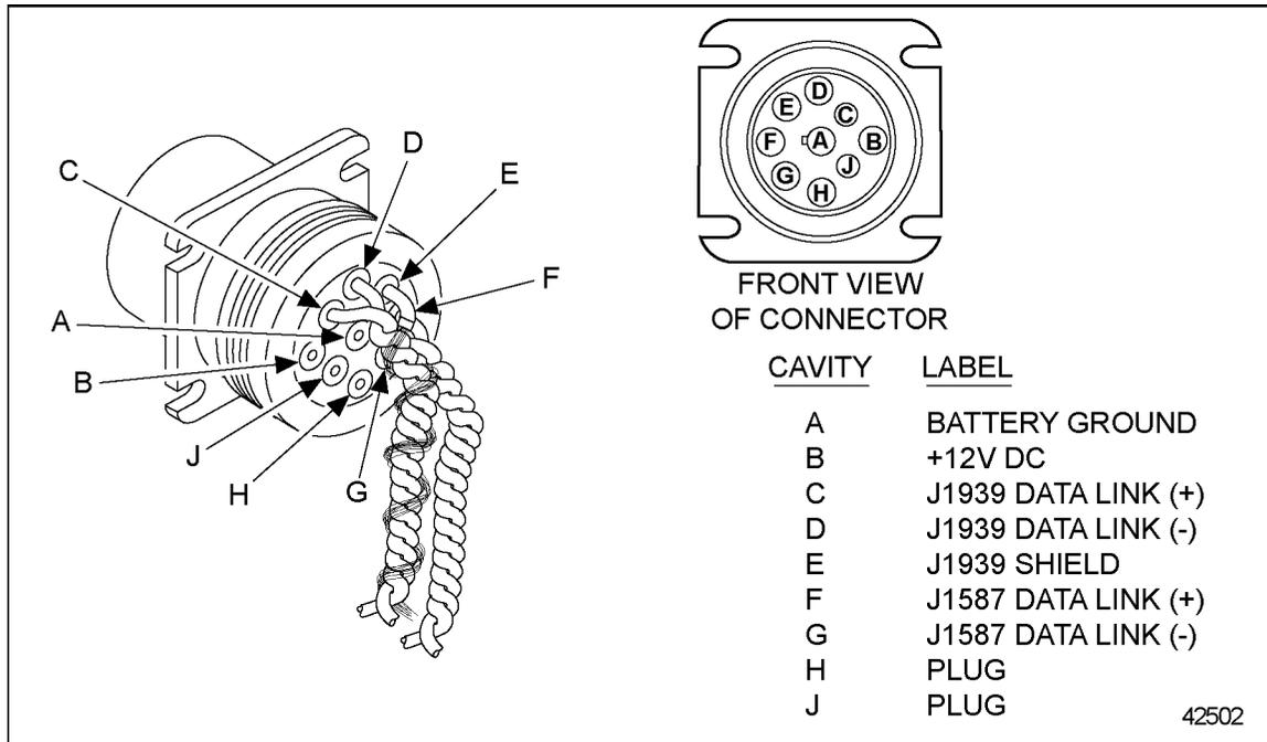
**Figure 3-13 Wiring for 9-pin Data Link Connector**
