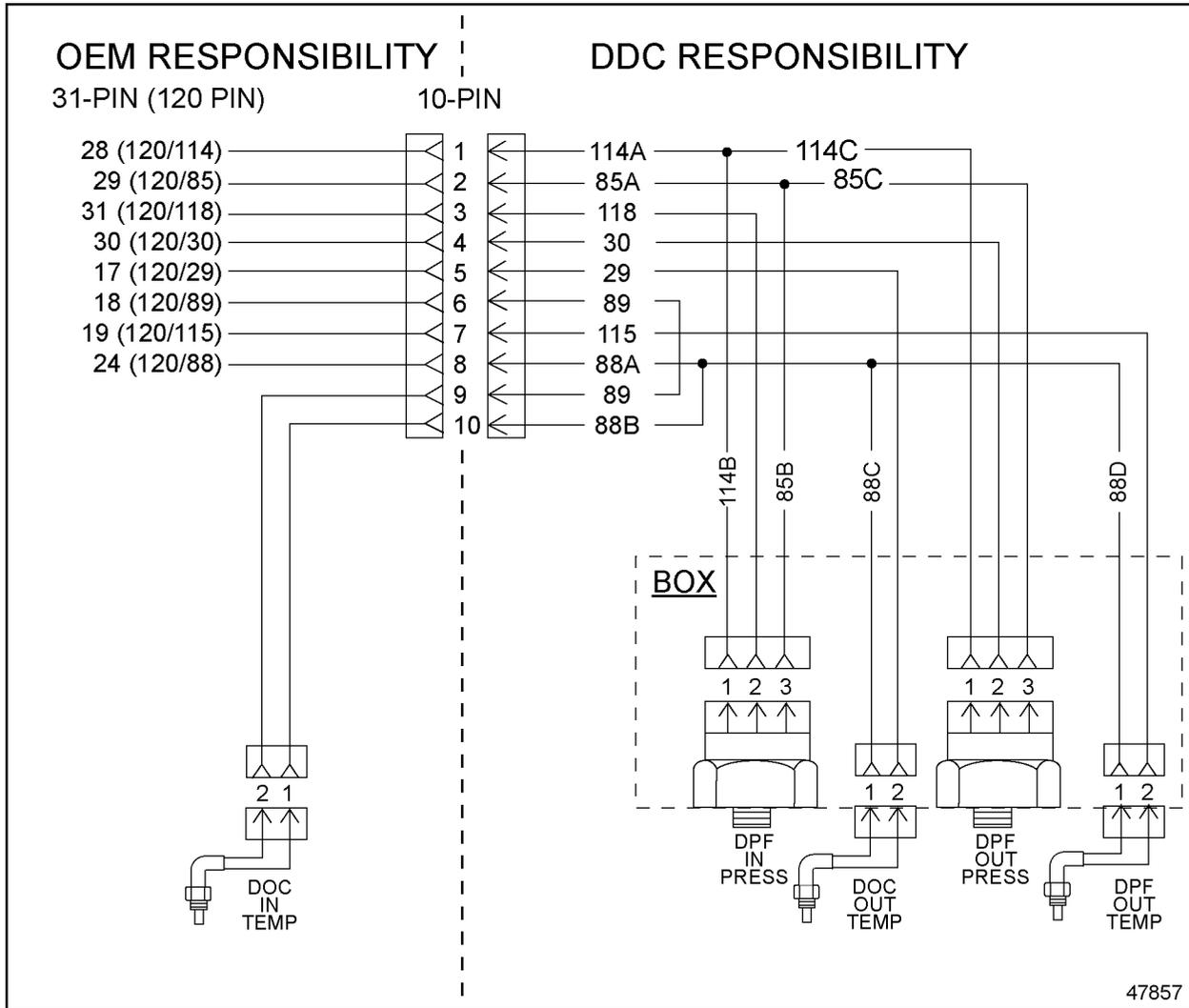
Figure 3-6 Horizontal Mount ATD Wiring — OEM Responsibility
