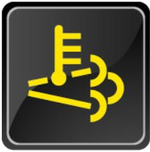
The HEST Lamp is controlled by DDEC VI.
