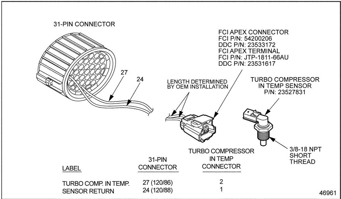
**Figure 3-32 Turbo Compressor In Temperature Sensor Installation**
