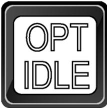
The Optimized Idle Active Lamp is controlled by DDEC VI..
