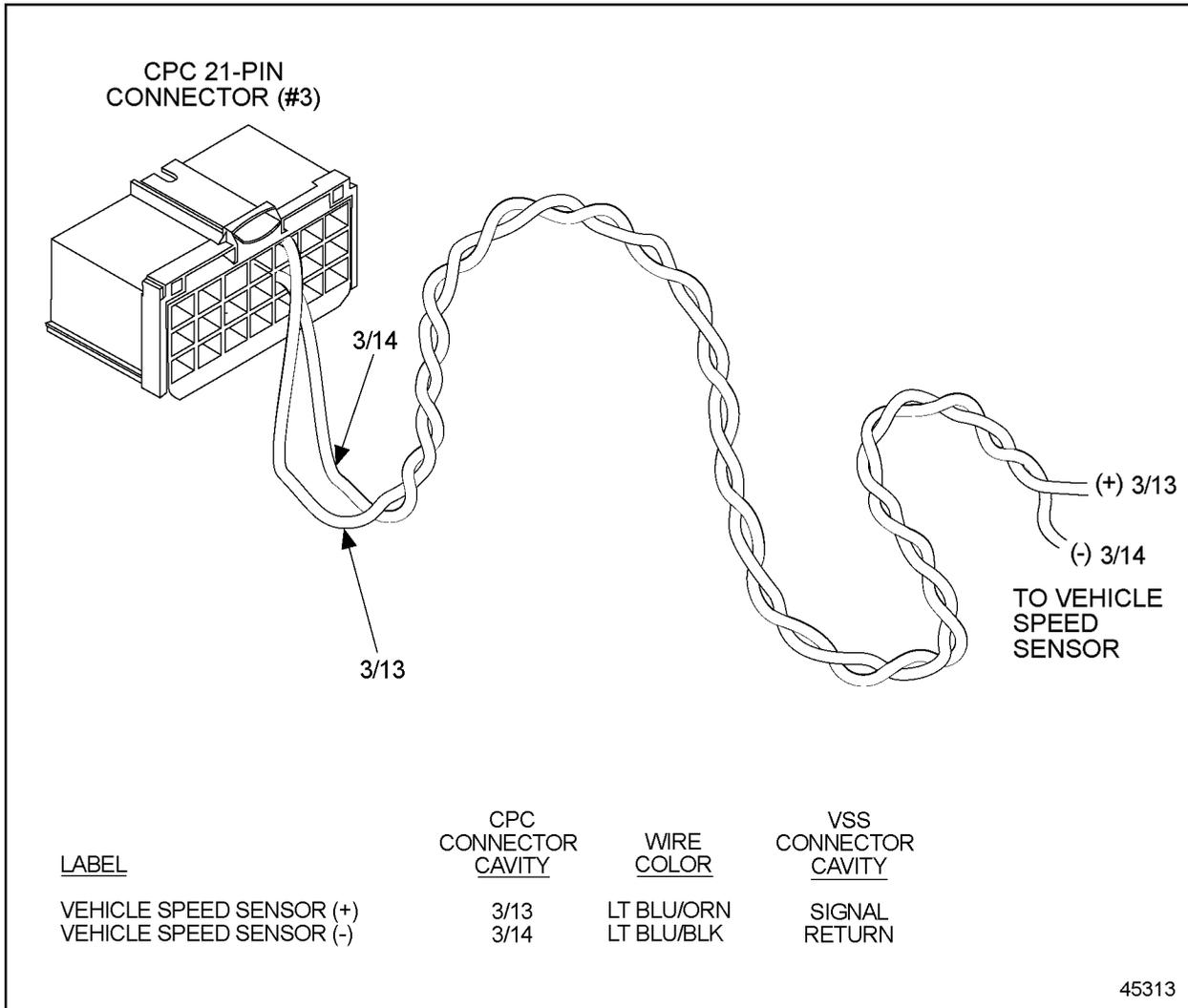
**Figure 3-34 Magnetic Vehicle Speed Sensor Installation – CPC**
