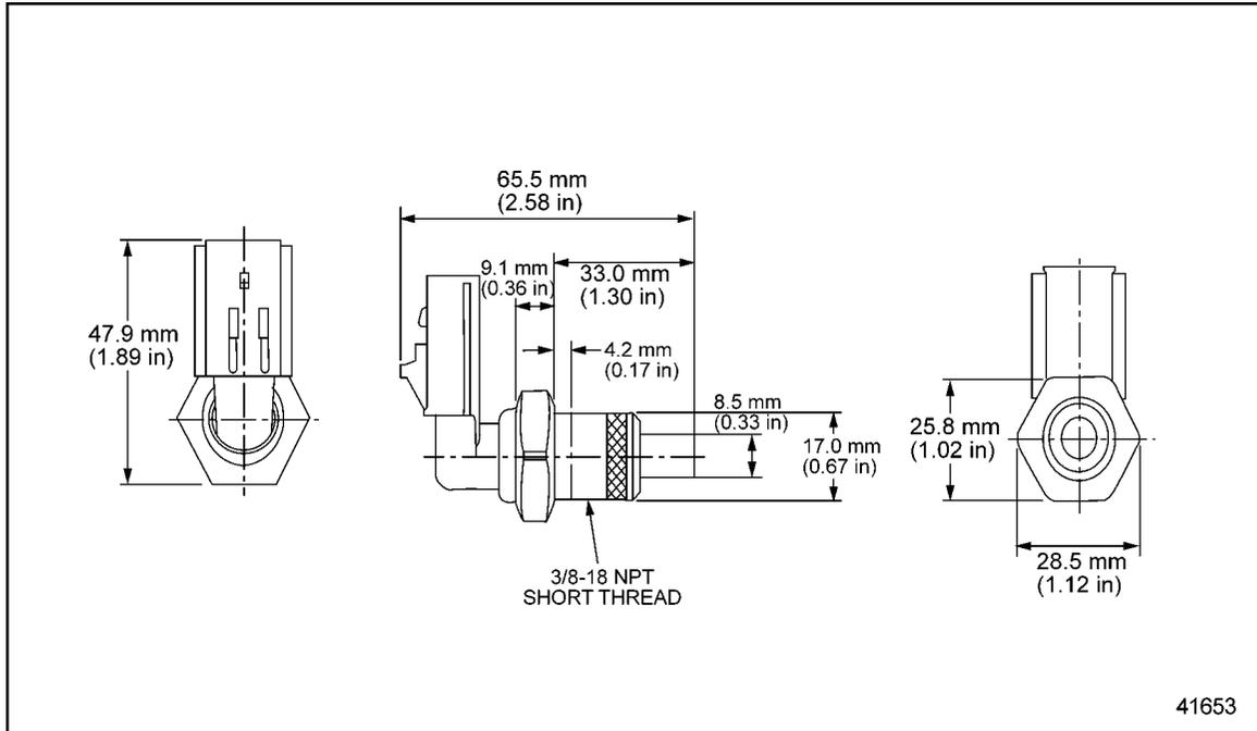
**Figure 3-31 Turbo Compressor In Temperature Sensor**
