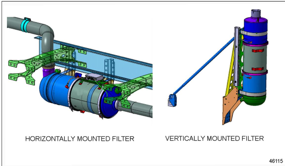
**Figure 3-4** Typical Mounting Views of an Aftertreatment Device
