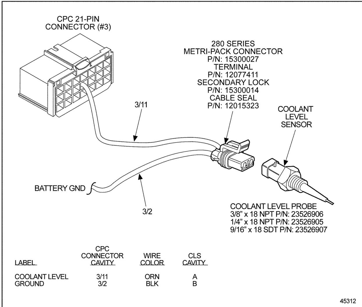
**Figure 3-29 Engine Coolant Level Sensor Installation for CPC**
