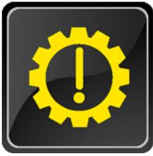
The AGS2 Check Trans Lamp is controlled by DDEC VI.
