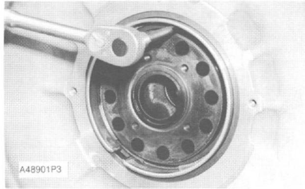
Removing Rear Wear Sleeve
