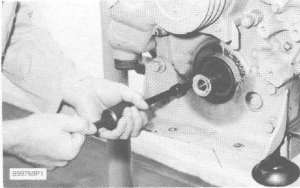
Removing Front Oil Seal
