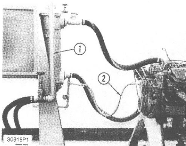
Shunt Line Connected To Engine
