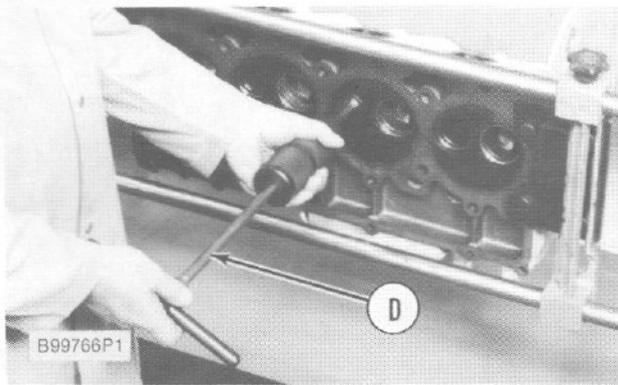
Removing Exhaust Valve Seat Insert
