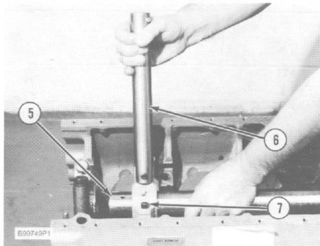
**Installing Bearing Assemblies**
