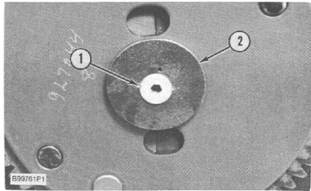
Removing Timing Advance Retaining Screw
