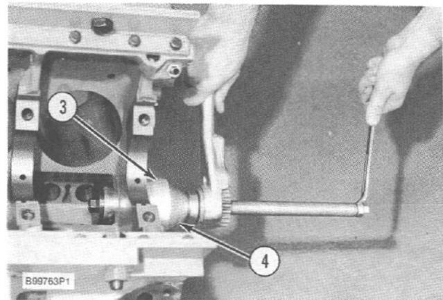
Installing Camshaft Front Bearing
