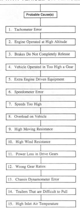
The problems in this chart are problems that do come about and are normally called "low power." These problems are not necessarily more common than engine problems, but they are possible problems which you need to read and check before an engine is disassembled.
