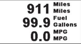
Setting up a Tank Minder is similar to an Odometer, but simpler. After selecting New Tank Minder and positioning it on the screen, right-click on the Minder and set the Tank Size. You can also customize the layout from this dialog box.
