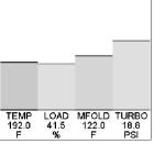
The MultiBar is customized very much like the Scan Gauge. Right-Click on the gauge to bring up the MultiBar Properties box. You may select as many parameters as you wish from the list at the top of the dialog box. You may choose whether to display the Gauge Name (the name is always abbreviated), the Value, and the Unit.
