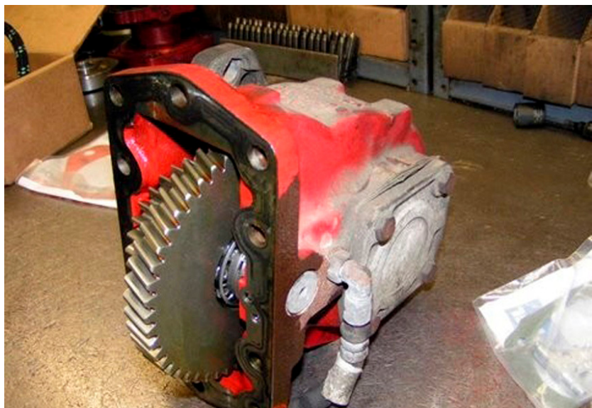
PTO showing single hose connection.
