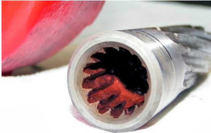
Close-up of old, worn output shaft, VERY close to failing.
