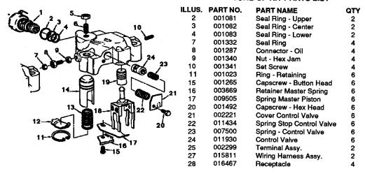
The parts in this kit are the most recent design by Jacobs, for the Model 71/92A and are Interchangeable with earlier production units. Follow the procedures outlined on this sheet. For complete information, refer to the Jacobs Engine Brake Installation Manual, Part No. 3879.
