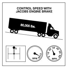
Under some circumstances, you may want to come down a grade at a faster rate than the control speed. This can be done by selecting a higher gear, or a lower position on the progressive braking switch. However, you may have to apply your service brakes intermittently to prevent overspeeding the engine and to keep the vehicle at a safe speed.
