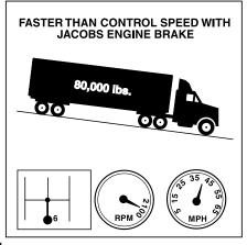
There may be circumstances in which you might want to descend a grade at a rate slower than the control speed. This is done by selecting a lower gear, one that will not overspeed the engine. You may have to apply the service brakes to obtain the desired lower speed.
