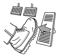
When you apply pressure to the throttle, the Jacobs Engine Brake is deactivated.
