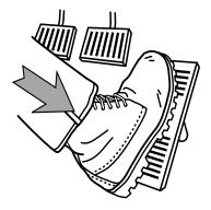
While shifting gears, the engine brake is automatically deactivated when you depress the clutch pedal.
