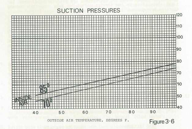
When the system is operating properly in warm weather, with the fan on high, the compressor should run warm to hot. The 3/8" or 1/2" suction copper tube and service valve should be cold and sweating. A warm suction service valve indicates too little gas. A cold compressor indicates too much gas.
