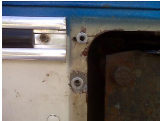
the main awning, getting rid of those sheet metal screws and installing Riv-nuts in their stead, thus not only sealing the top edge of the awning rail but sealing, fully, the screw entry holes completely that are along the roof line.
