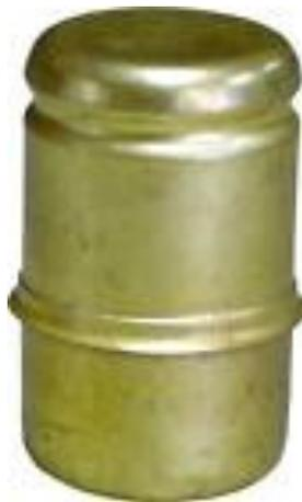
The photo of the in fuel tank sending unit is the typical style in our Coaches and the brass float is the normal thing to find. Note the 1/2 circle on the end of the arm of the sender, then note the detent on the brass float. The float simply snaps into place on the old sender arm already in the tank.
