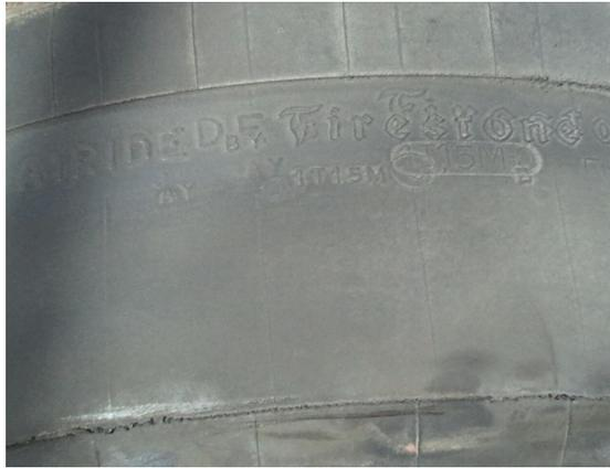
the Coach rests upon when the suspension is dumped. The steel plate that forms the top of the Air Spring is the opposite resting place.
