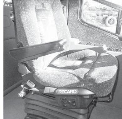
The seat should be adjusted appropriately for the individual operator. Adjustments should be made not only for comfort, but for optimum visibility and full access to bus controls. Control buttons for seat height and tilt, back tilt, and lumbar support are provided on a convenient control panel on the right side of the Recaro seat. These adjustments are air-actuated. Thus, the auxiliary tanks of the bus's air system must be pressurized in order for these seat controls to operate.
