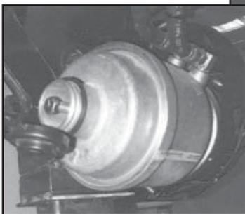
Figure 48 - Brake Release Tag Axle
