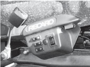
The seat should be adjusted appropriately for the individual operator. Adjustments should be made not only for comfort, but for optimum visibility and full access to bus controls. Control buttons for seat height and tilt, back tilt, and lumbar support are provided on a convenient control panel on the right side of the Recaro seat. These adjustments are air-actuated. Thus, the auxiliary tanks of the bus's air system must be pressurized in order for these seat controls to operate.
