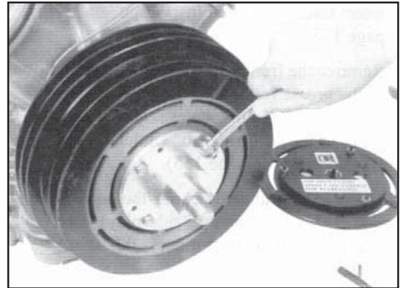
Figure 92: Securing Collar to Pulley
