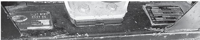
**The Body Serial and Service Number Plate** is located on the defrost plenum front flange. Refer to the data on this plate for registration purposes or for replacement part information pertaining to the bus body.
