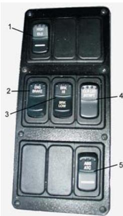
1. **HIGH IDLE** – When a higher idle speed is needed, the engine can be placed in the high idle by:
