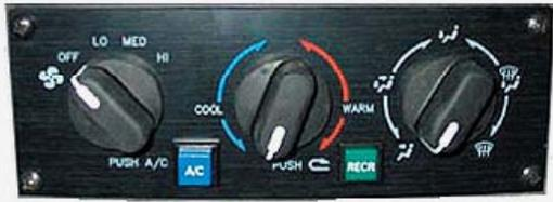
The first dial on this panel lets the user select between Fan, Off, Lo, Med, and Hi speed for either the heater or the air conditioner. The second button chooses between cool and warm air. The third button controls where the air or heat will be directed. These are much like the standard controls that come with any vehicle. To select air conditioning, push the blue AC button at the bottom of the panel. To choose recirculating air push the green RECR button located on the bottom of this panel.
