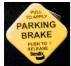
Figure 45 - Parking Brake Valve
