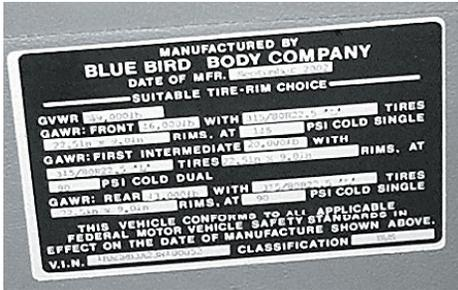
**The Vehicle Certification Plate** is located on the auxiliary shifter cabinet below dash at front leading edge. This plate provides Gross Vehicle Weight Ratings, specifies tire inflation pressures, and certifies that the vehicle conforms to all applicable Federal Motor Vehicle Safety Standards in effect at the date of manufacture. Do not remove or deface this plate.
