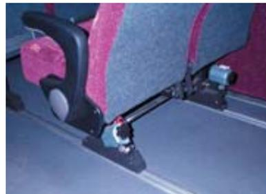
Regular seat inspection and maintenance is an important part of the operation regimen for vehicles used for passenger transport. At least every 90 days, inspect and retighten all bolts, and inspect upholstery for cuts and tears. Repair or replace as needed. Express 4500 seats are equipped with a special foam back pad. If the pad becomes damaged, it should be replaced with an approved replacement part. Any aftermarket replacements should be checked for compliance with Federal standards.
