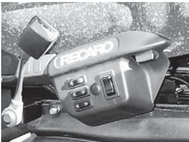
Other controls on the seat are mechanical, and therefore require no air pressure for operation. Individual controls for left and right armrest height are adjusted by knobs under the front end of each armrest. Fore and aft adjustment of the seat is also mechanical, and is accomplished by lifting the lock lever at the front underside of the seat cushion. For more information, refer to the Recaro documentation provided with your unit.
