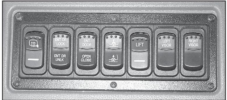
As indicated by the icon on the switch, pressing the switch downward kneels the bus. Air is released from the front air suspension bags very rapidly, allowing the entrance door step to drop three inches in three seconds. The horn sounds as a warning and a yellow indicator appears in the instrument panel.
