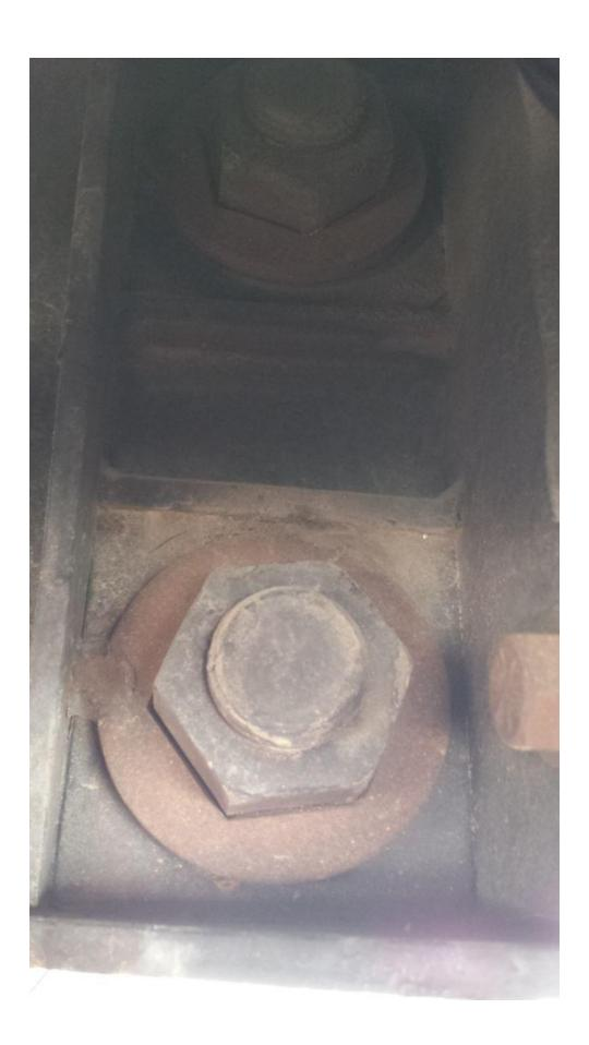
Grind through the welds on the nut end.
